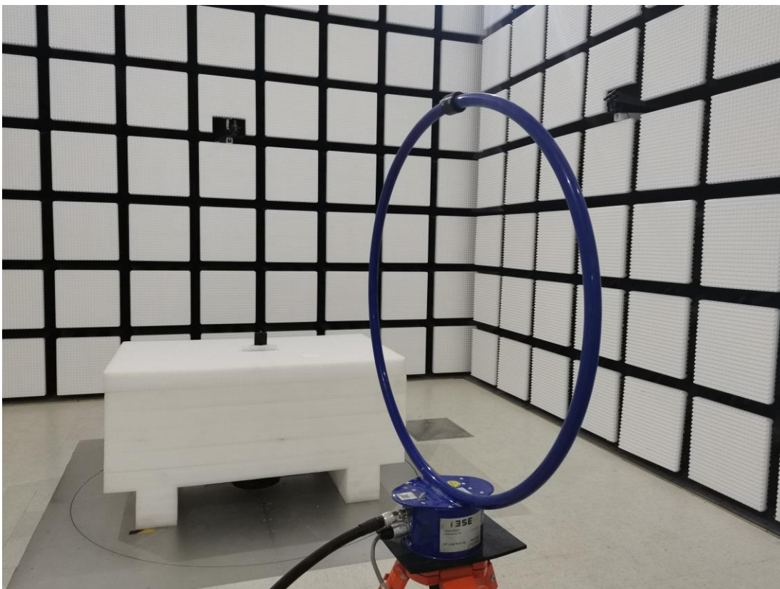
Radiated Emission 9kHz - 30MHz Perpendicular View
