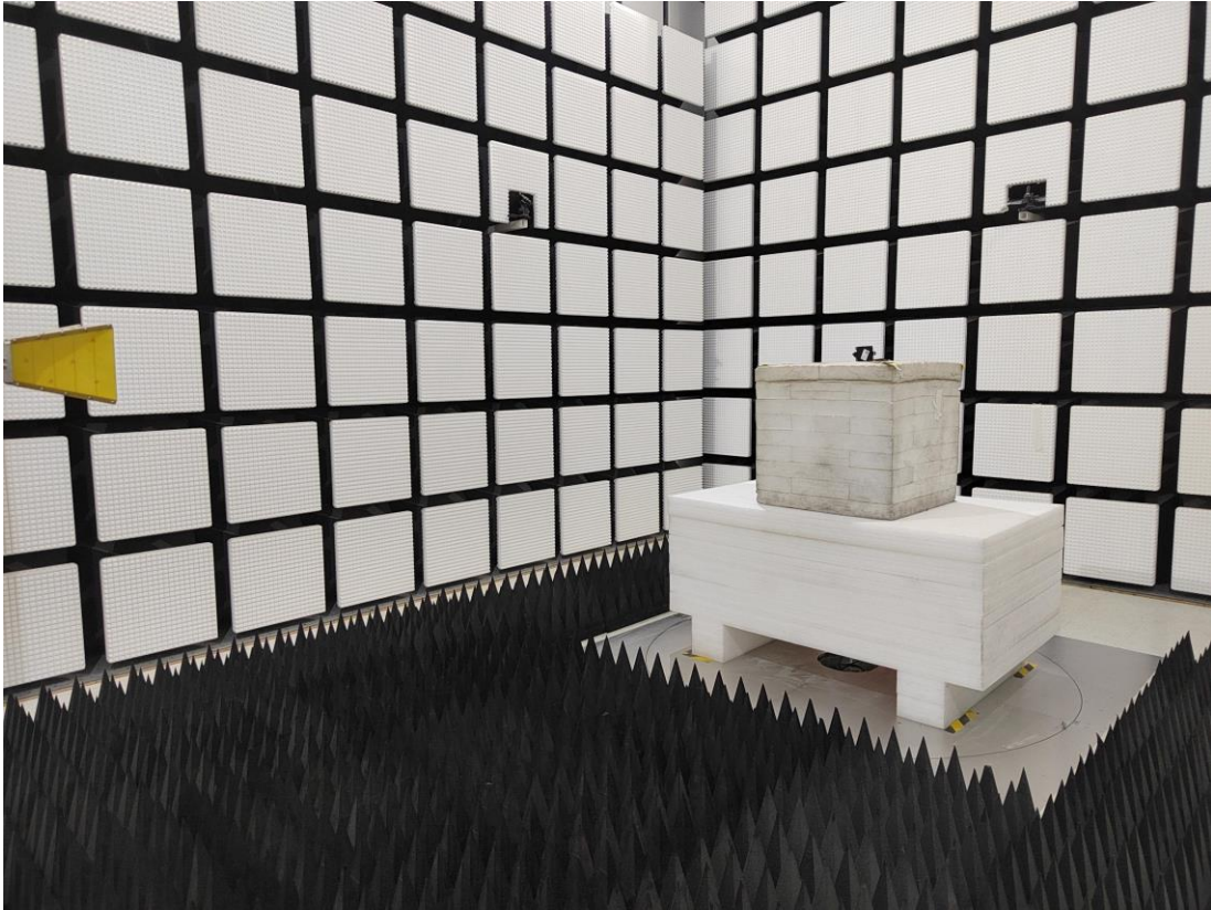
Radiated Emission Above 18GHz - 26.5GHz View
