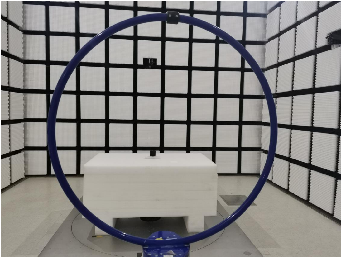
Radiated Emission 9kHz - 30MHz Perpendicular View
