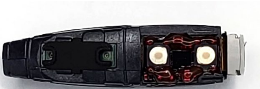
Internal photo of hearing aid with antenna, Top view
