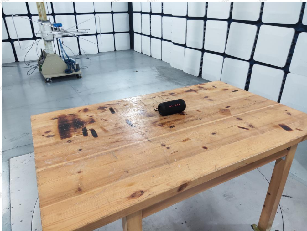
Photo of Radiation Emission Test
