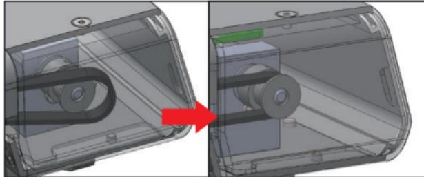
The timing belt covers the timing wheel. **R**
