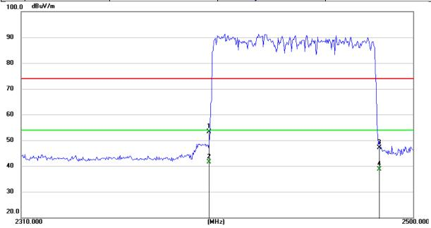
Spurious Emission in Restricted Band 2310-2390MHz and 2400-2483.5MHz
