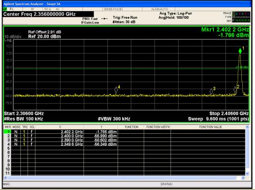
Maximum Conduceted Level RBW=100kHz
