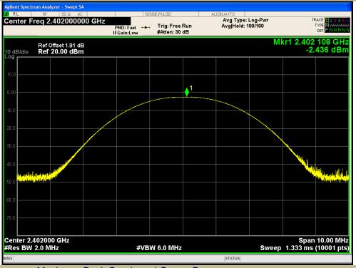
Maximum Peak Conducted Output Power Test Model Bluetooth V5.3
