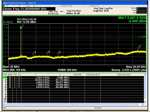
Maximum Conduceted Level RBW=100kHz
