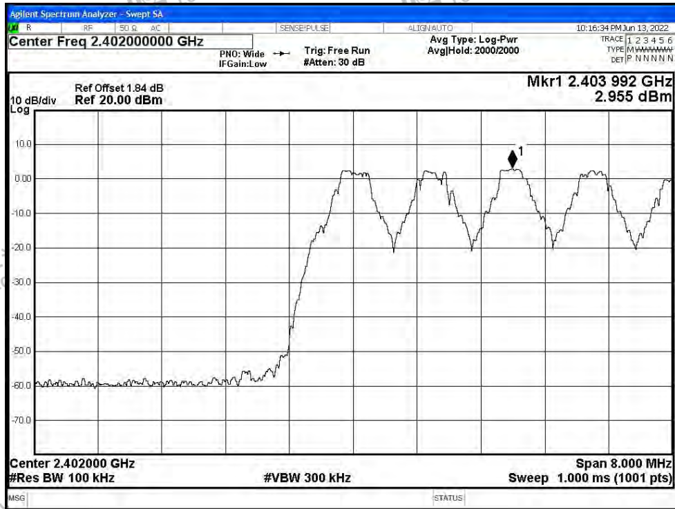
Band Edge(Hopping) NVNT 1-DH5 2402MHz Ant1 Hopping Emission
