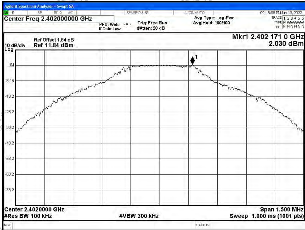
Tx. Spurious NVNT 1-DH5 2402MHz Ant1 Emission
