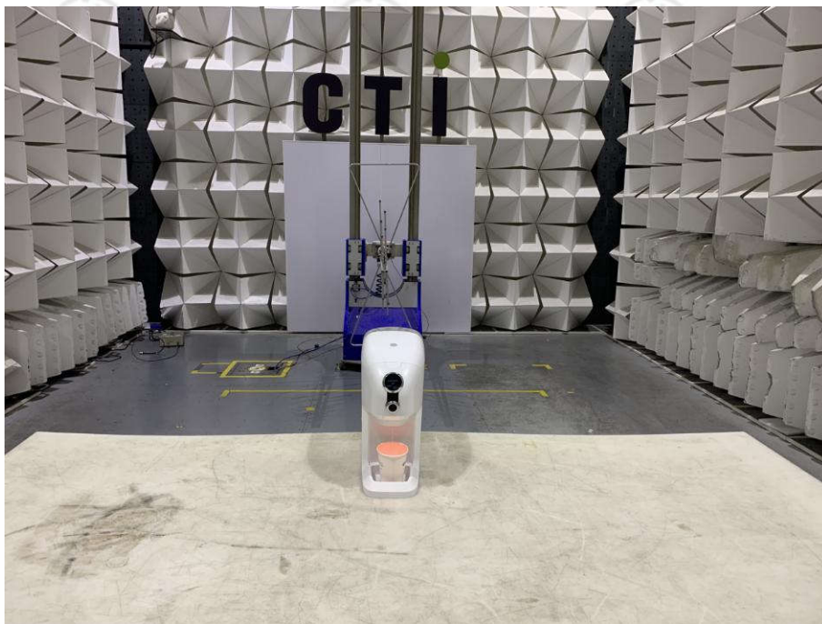
Radiated spurious emission Test Setup-1(Below 1GHz)
