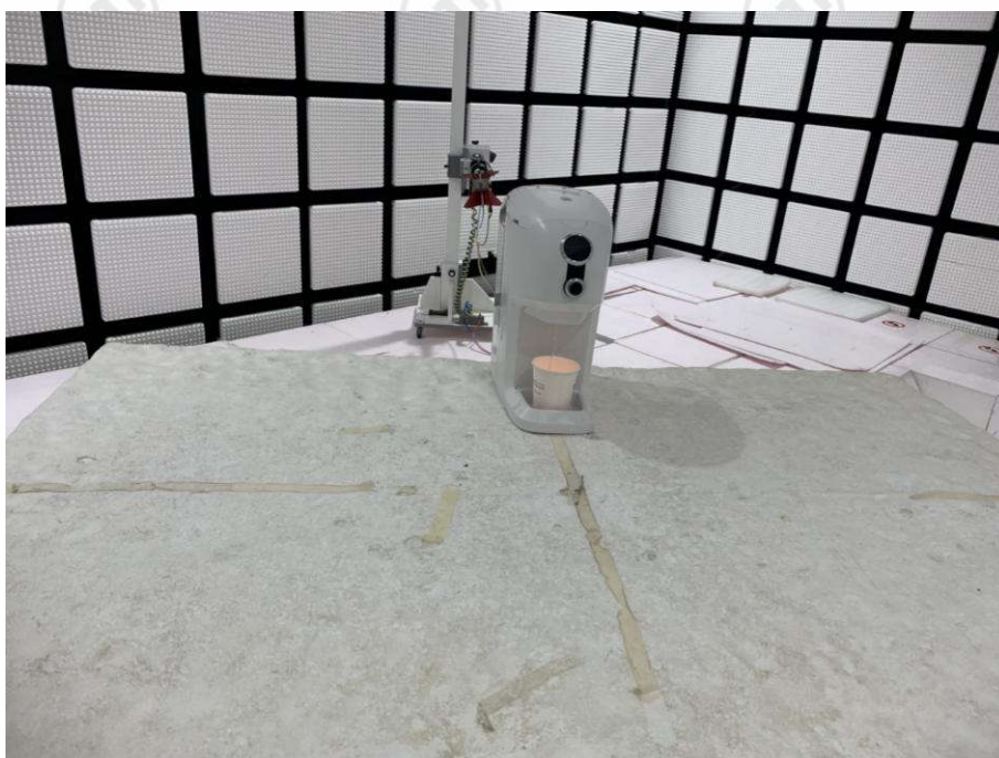
Radiated spurious emission Test Setup-2(Above 1GHz)
