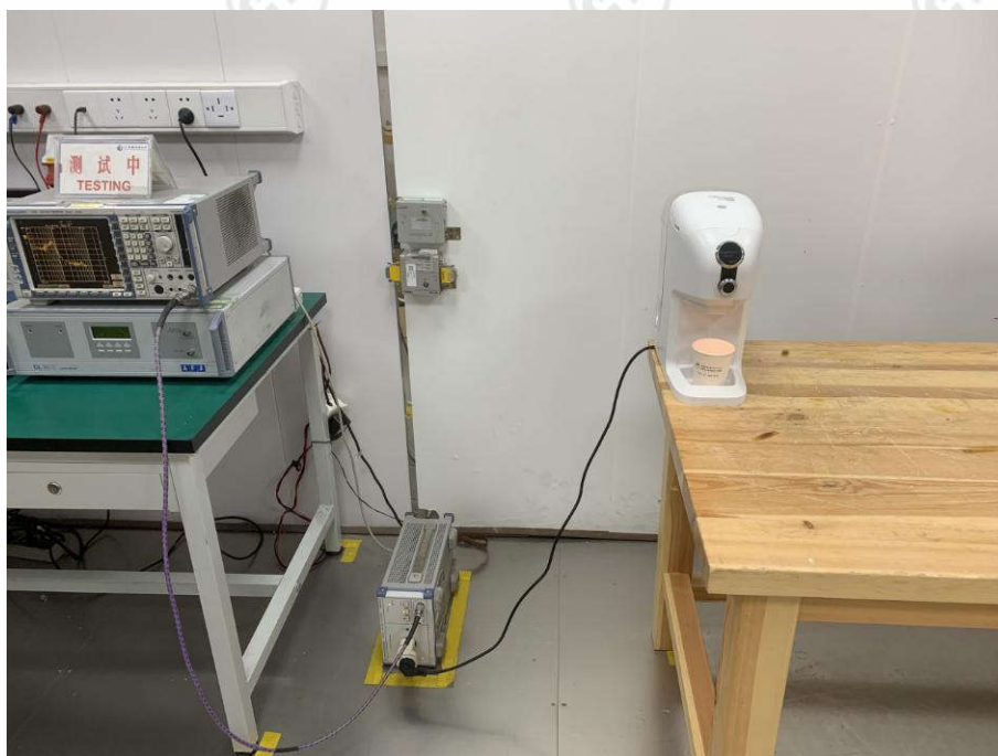
CONDUCTED EMISSION TEST SETUP
