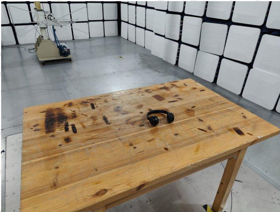
Photo of Radiation Emission Test
