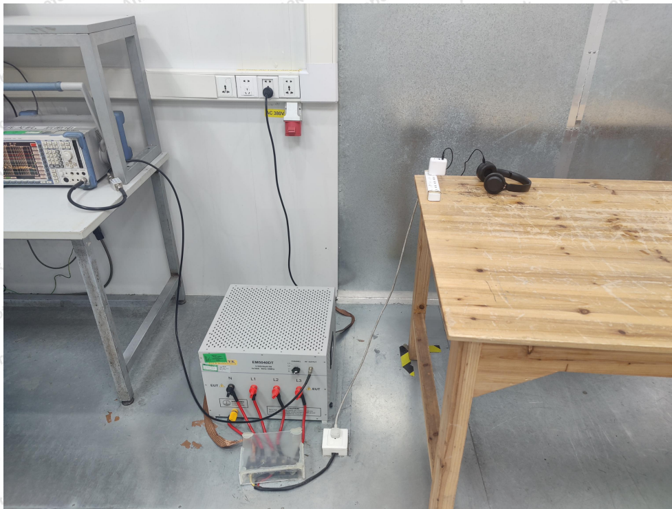
Photo of Conducted Emission Measurement
