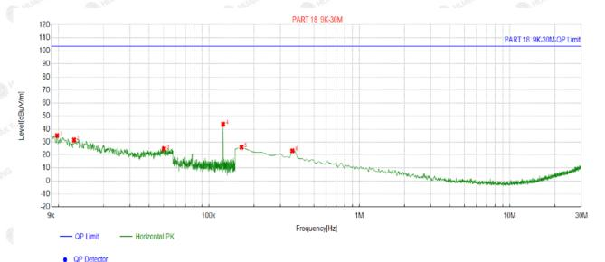
Suspected List Factor Reading Level Limit Freq. Margin NO. [dBµV/m] [MHz] [dB] [dBµV/m] [dBµV/m] [dB] 1 0.0098 -14.14 49.18 35.04 103.50 68.46 0.0127 -14.99 46.59 31.60 103.50 71.90 2 3 0.0503 -17.1541.94 24.79 103.50 78.71 4 0.1244 -17.2361.00 43.77 103.50 59.73 5 77.47 -17.30 43.33 26.03 103.50 0.1649 6 0.3591 -17.2240.41 23.19 103.50 80.31
