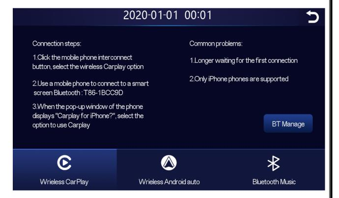
As shown in the figure above, click the [Mobile Phone Internet] button to enter the wireless carplay and wireless Android AUTO selection, click the [Bluetooth Management] option of the interface, and connect to Bluetooth with the mobile phone, you can open the application.
