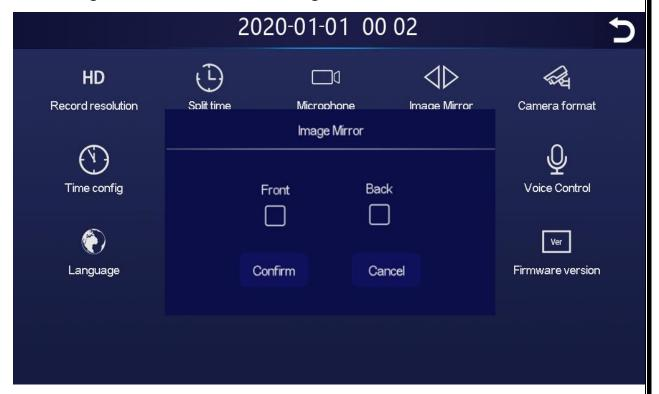
The system can mirror the front / rear view camera separately.
