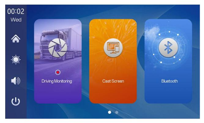
As shown in the figure above, the camera image will not be displayed in the main page, and the camera image needs to click the [dashcam] button to view. When a card is inserted, the system automatically enters the video mode, and when recorded, the small red dots in the [dashcam] button will flash.
