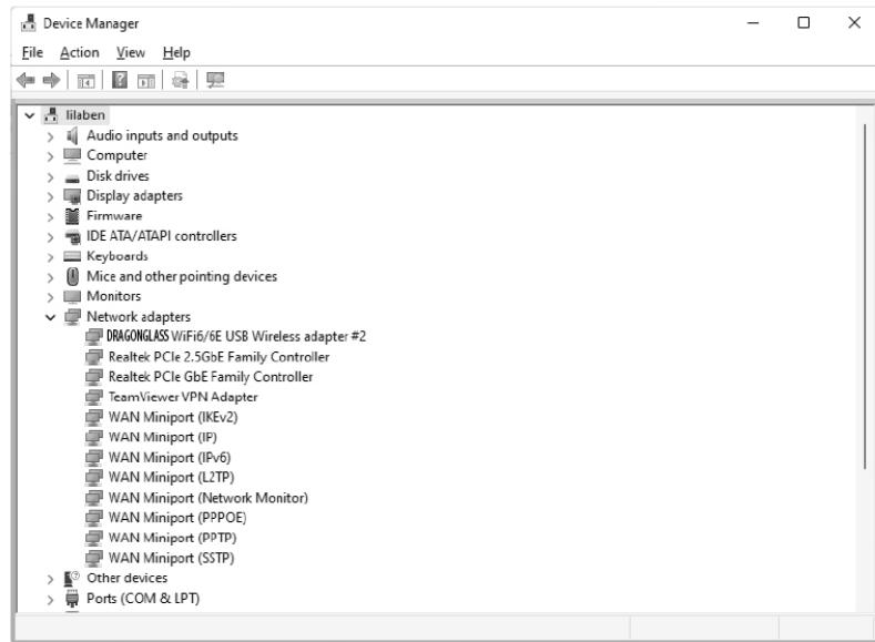
**2-6 Double-click to view the device details. If there is no abnormality, the driver is running normally as shown in the figure below and the driver details can be viewed;**
