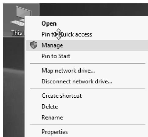
**2-5 After entering the management page, click Device Manager, Network Adapter in turn, you can see the installed network card driver (Note: This step requires the network card to be connected to the computer to see it.)**
