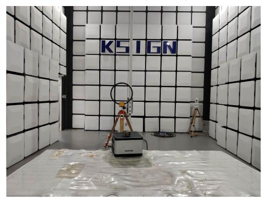
Radiated Measurement (Above 30MHz)
