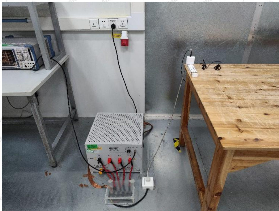
Photo of Conducted Emission Measurement
