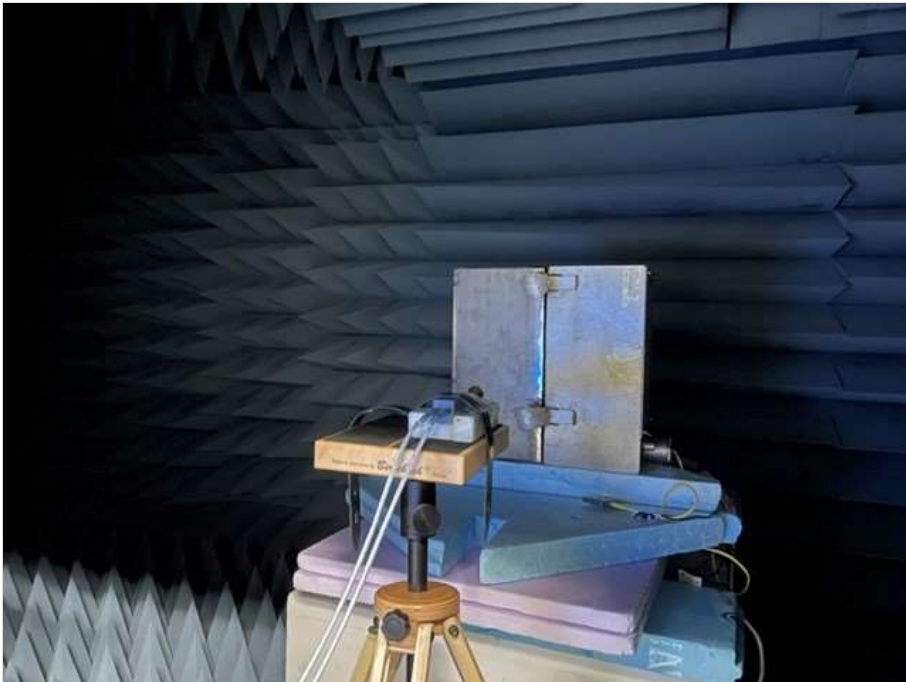
Photograph 6: EUT test setup in the fully anechoic chamber, close up view_EUT elevation 90°
