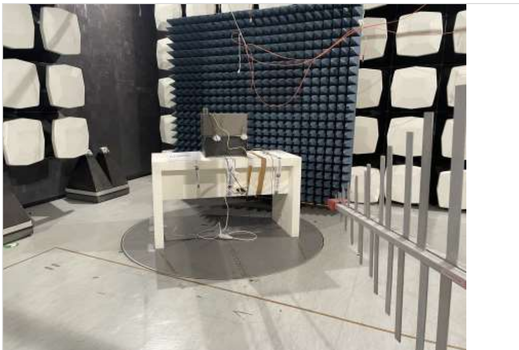
Photograph 5: EUT test setup in the semi anechoic chamber, overview
