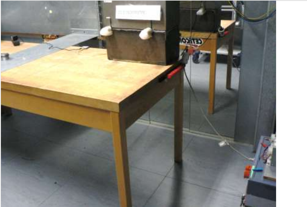
Photograph 1: EUT setup conducted measurement, over view
