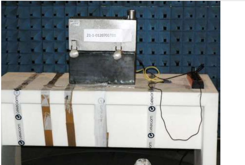
Photograph 2: EUT test setup in the semi anechoic chamber, close up view, magnetic field measurements
