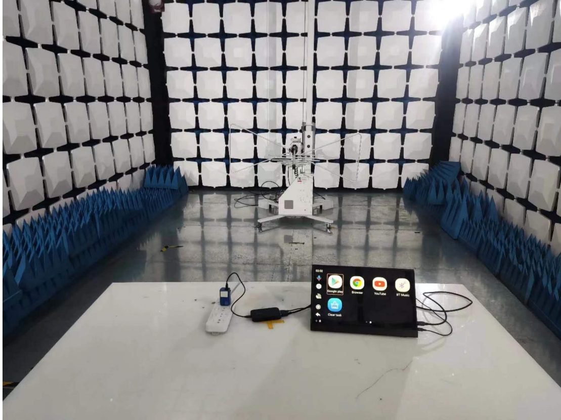
Above 1GHz for radiated emission test setup
