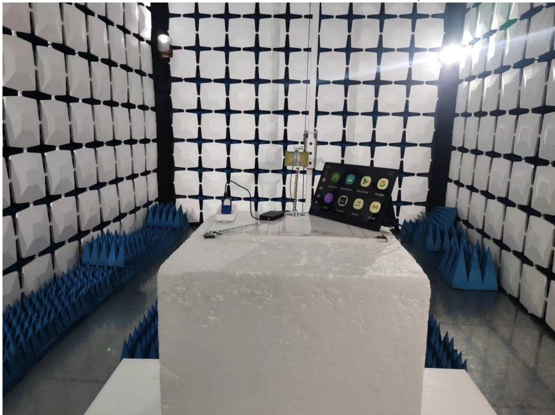
Above 1GHz for radiated emission test setup
