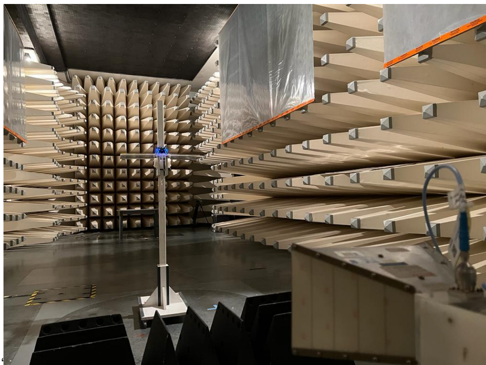
Set-up for Radiated Emission (1GHz above)
