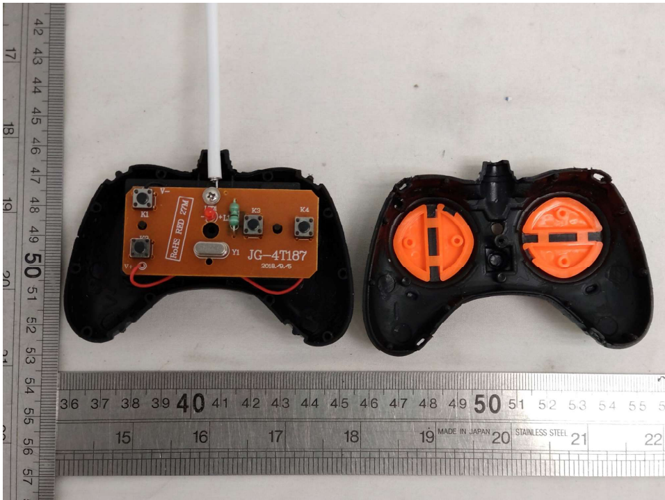
Transmitter (Internal view)
