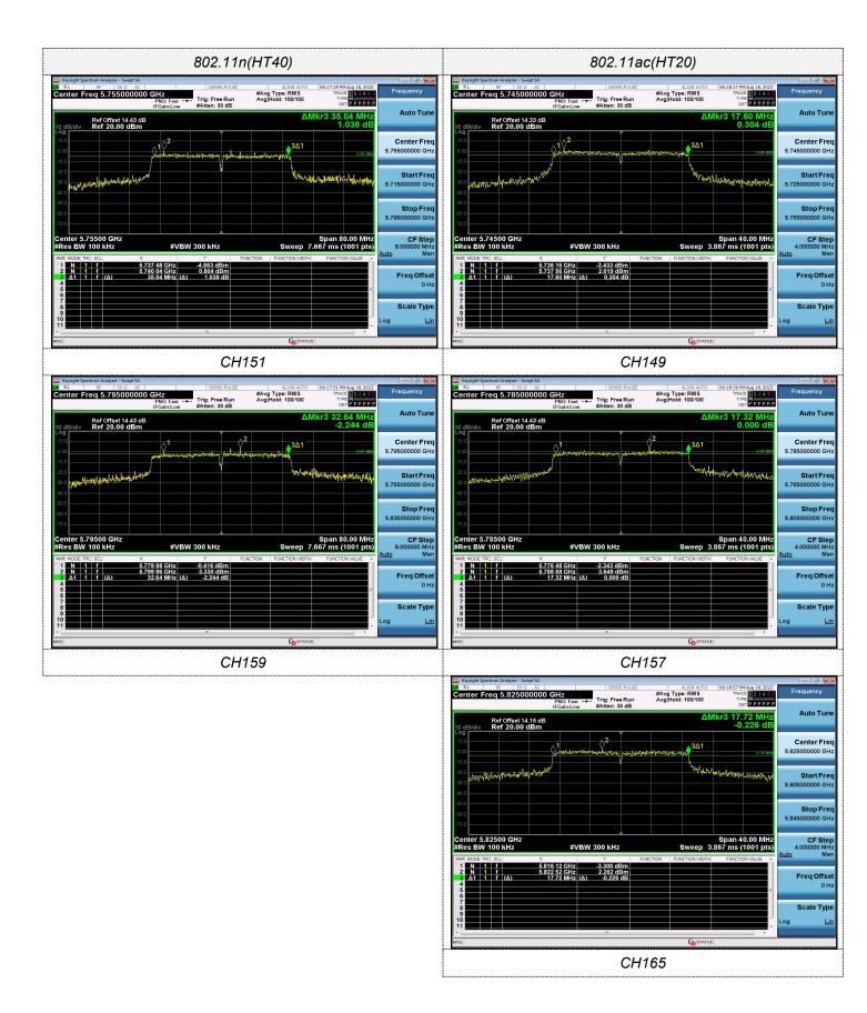
5.777 48 GHz 0.451 dBm 5.807 48 GHz 3.314 dBm 34.40 MHz (Δ) -3.006 dB
