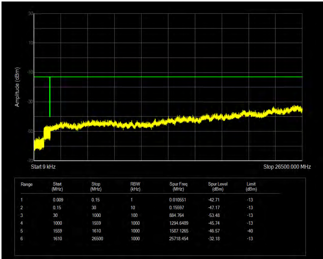
Band13 16QAM BW=5MHz Channel=23255 RB Size=1 Position=#0
