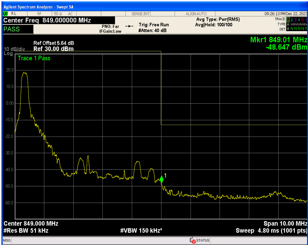
Band5 16QAM BW=5MHz Channel=20425 RB Size=25 Position=#0
