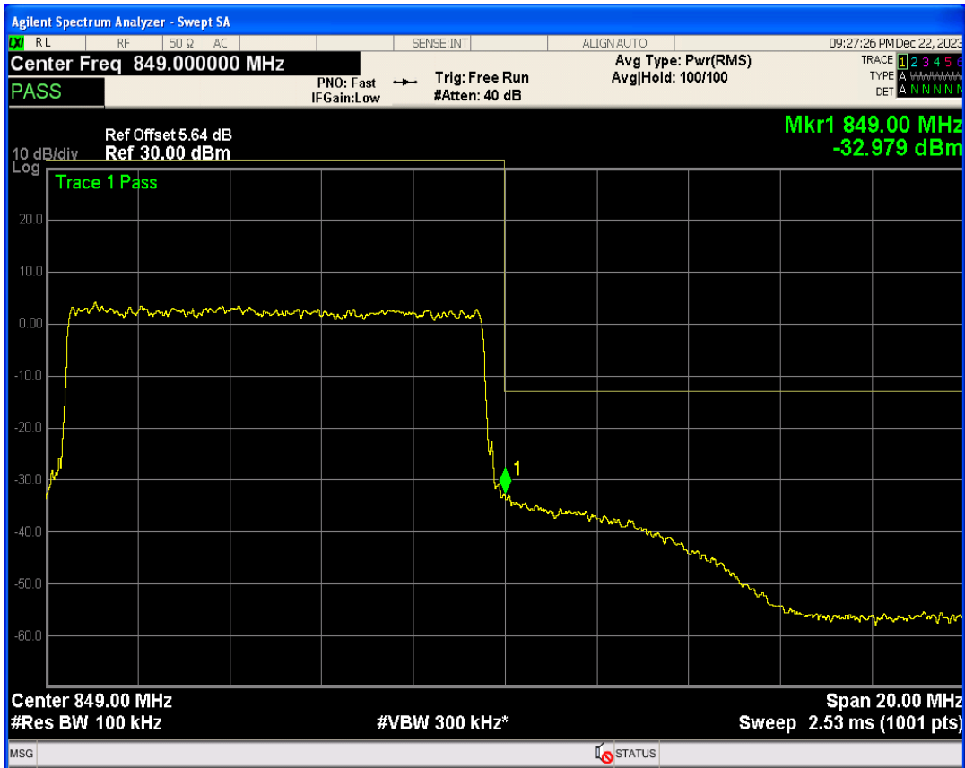
Band66 QPSK BW=1.4MHz Channel=131979 RB Size=1 Position=#0
