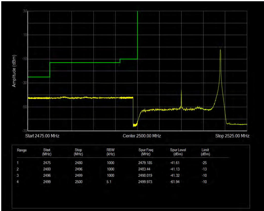
Band7 QPSK BW=20MHz Channel=20850 RB Size=100 Position=#0
