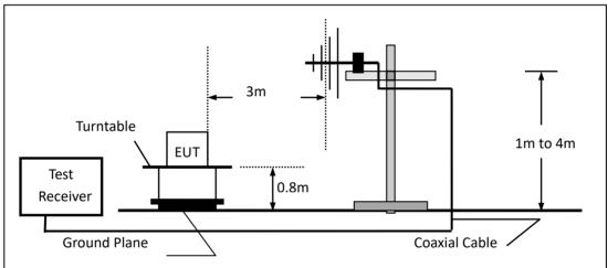
(c) For radiated emissions above 1000MHz
