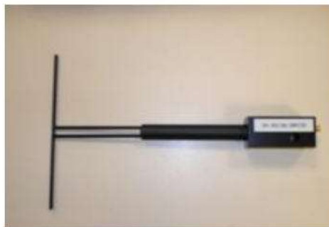
Figure 1 – Satimo COMOSAR Validation Dipole
