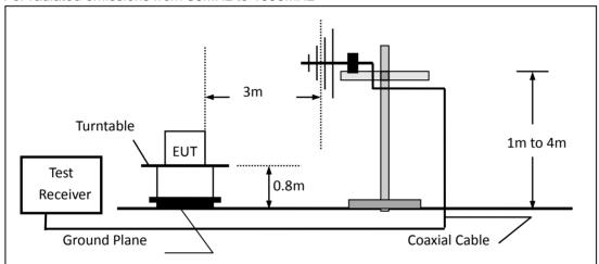
(c) For radiated emissions above 1000MHz
