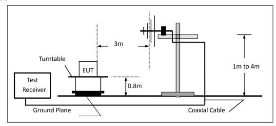
(c) For radiated emissions above 1000MHz
