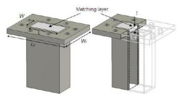
Figure 1: Validation Waveguide Dimensions
