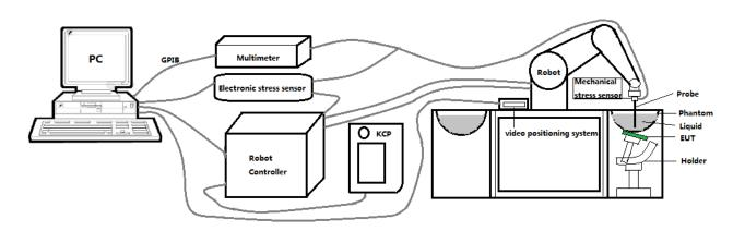
These measurements were performed with the automated near-field scanning system OPENSAR from SATIMO. The system is based on a high precision robot (working range: 901 mm), which positions the probes with a positional repeatability of better than  $\pm 0.03$  mm. The SAR measurements were conducted with dosimetric probe (manufactured by SATIMO), designed in the classical triangular configuration and optimized for dosimetric evaluation.
