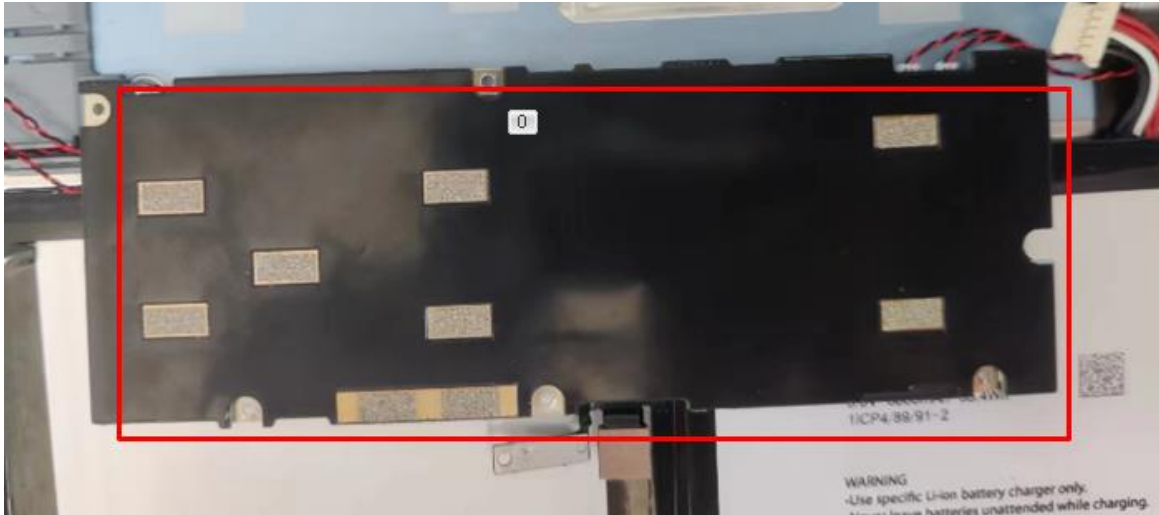
Figure: The red box is grounded with conductive cloth.
