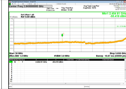
Spurious Emission:30.0~5650 MHz IEEE 802.11n_Channel 157_20MHz_Antenna 0
