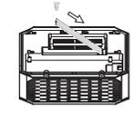
1. Open the groove of SD card with the hex key (M2.5) for the motherboard.
