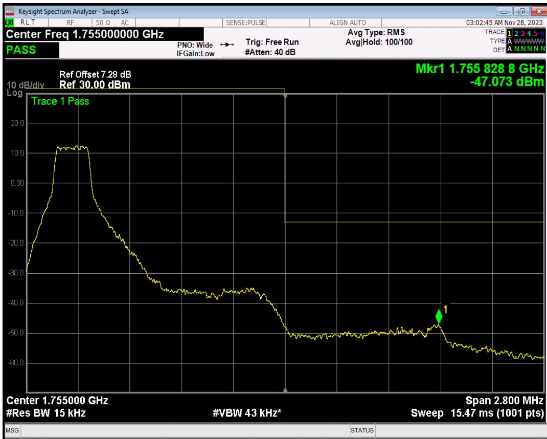
Band4 16QAM BW=1.4MHz Channel=20393 RB Size=1 Position=#Max
