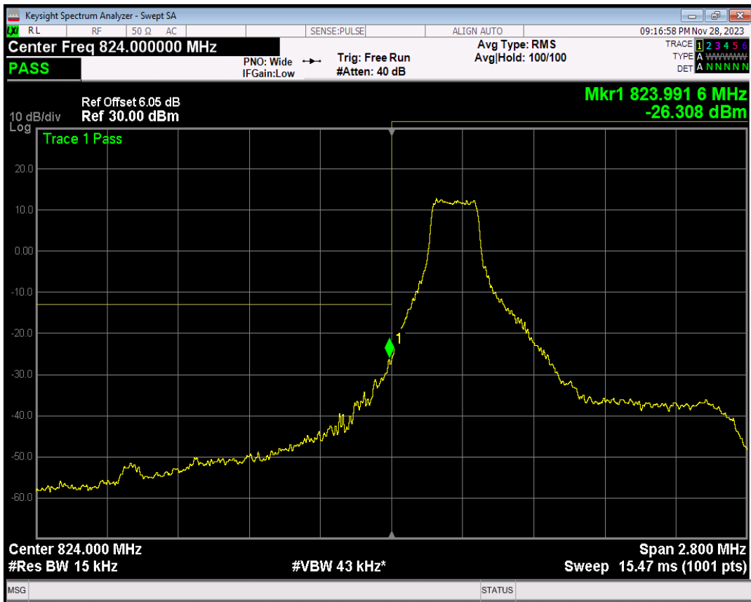
Band5 16QAM BW=1.4MHz Channel=20407 RB Size=1 Position=#Max
