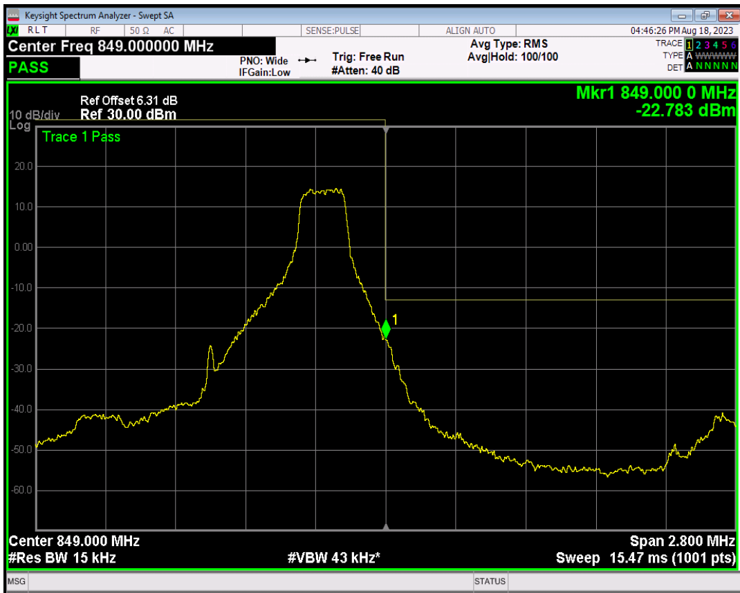
Band5 QPSK BW=1.4MHz Channel=20643 RB Size=6 Position=#0
