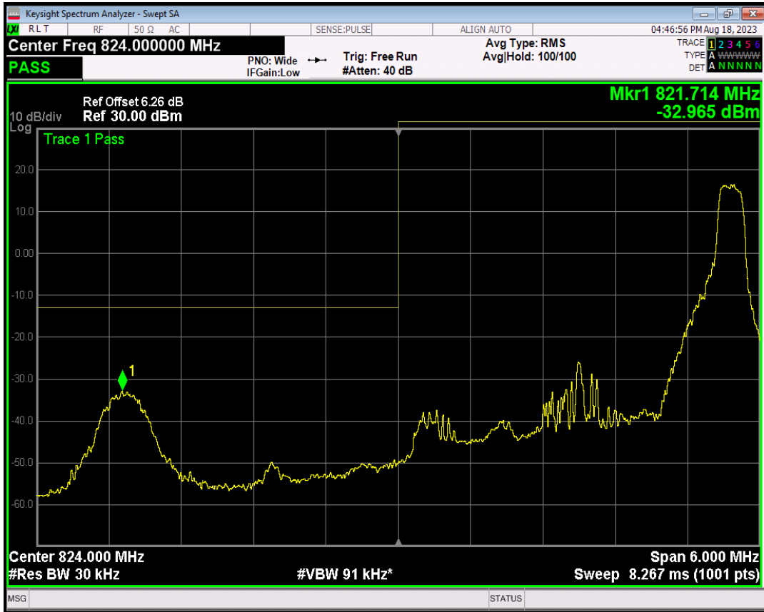
Band5 16QAM BW=3MHz Channel=20415 RB Size=15 Position=#0
