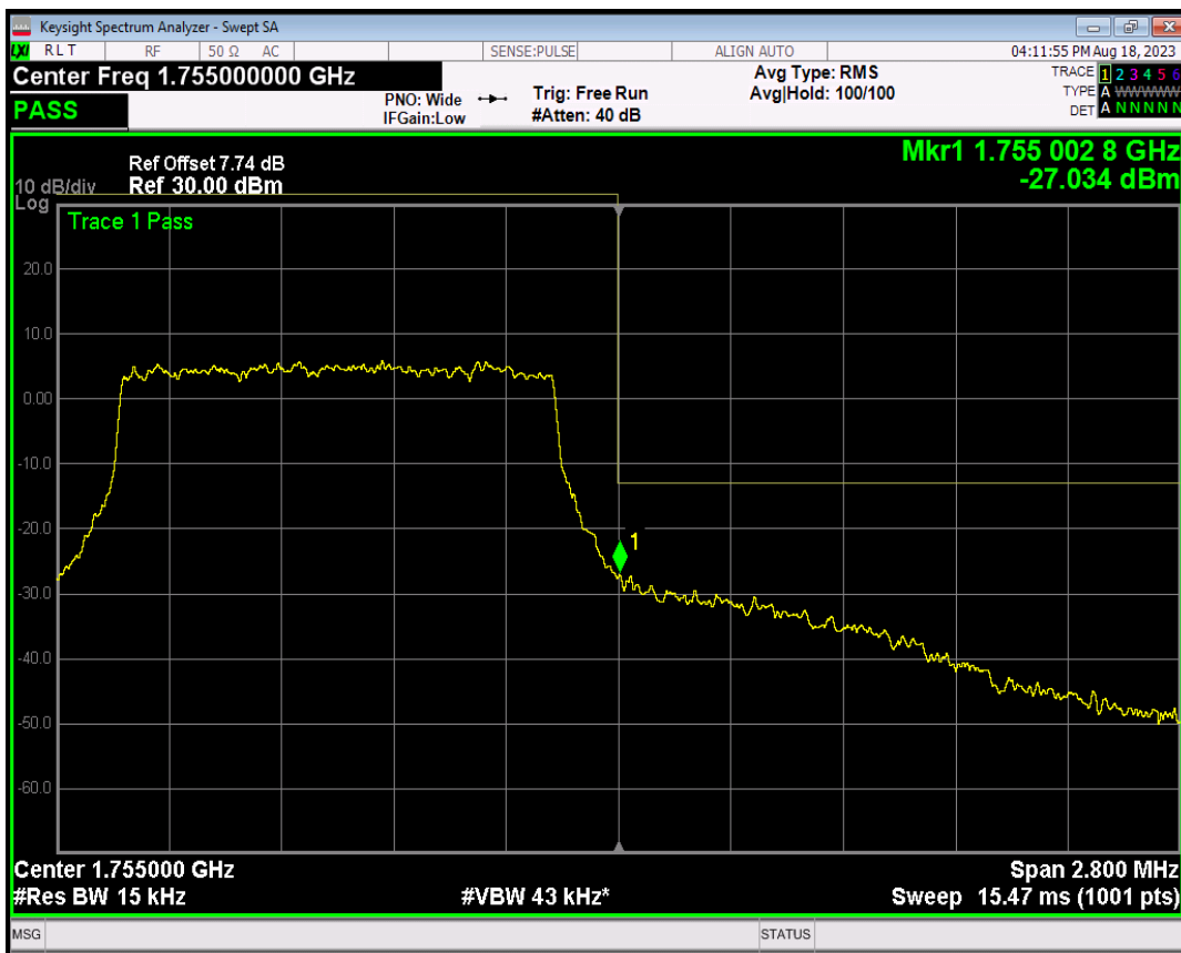
Band4 QPSK BW=3MHz Channel=19965 RB Size=1 Position=#0
