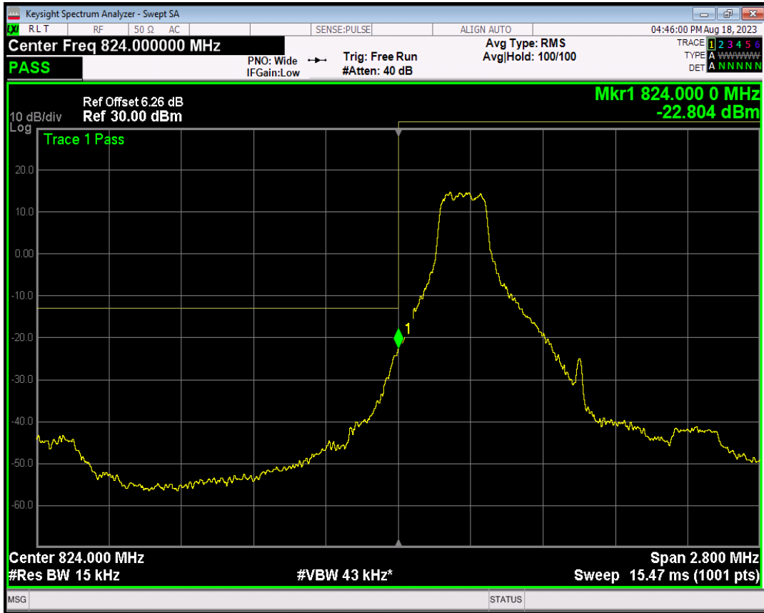
Band5 QPSK BW=1.4MHz Channel=20407 RB Size=1 Position=#Max
