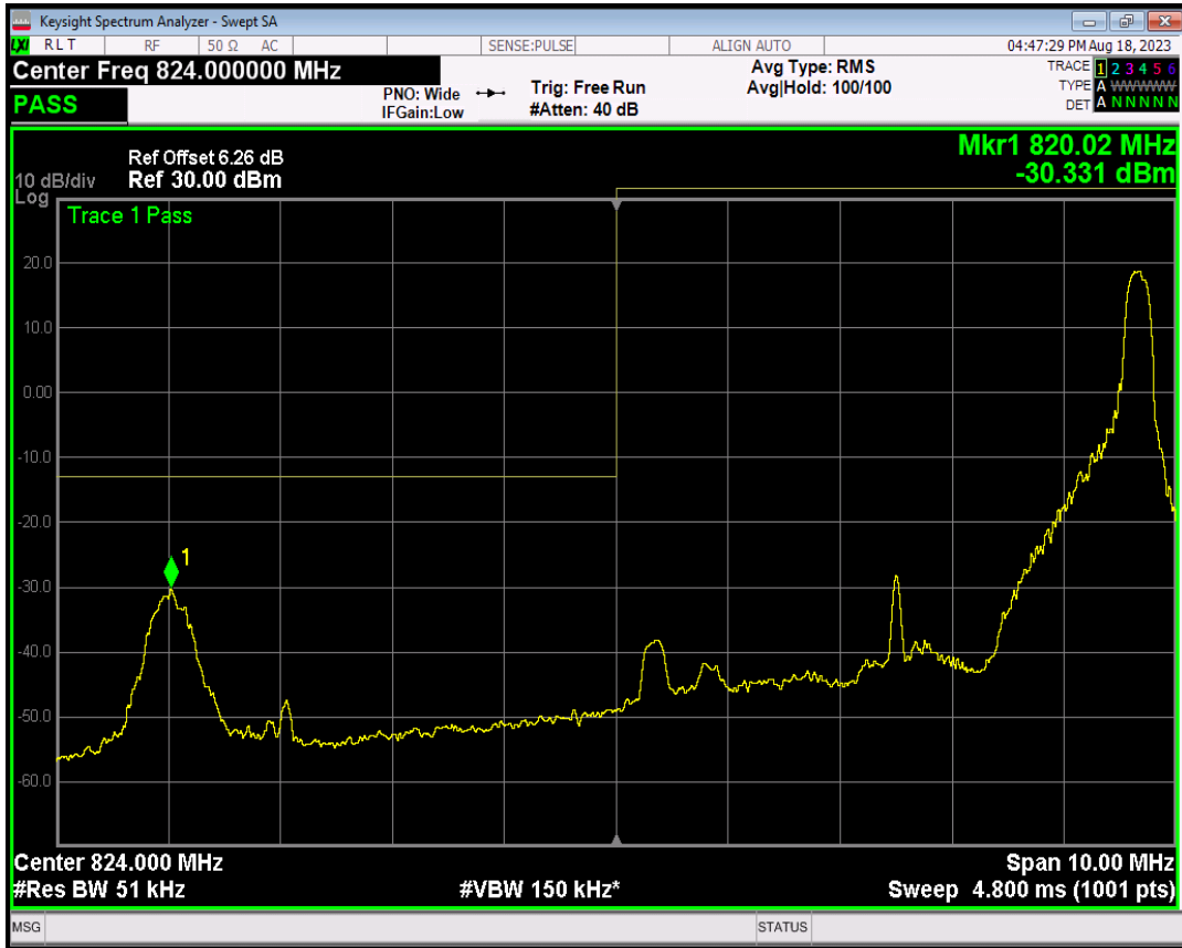
Band5 QPSK BW=5MHz Channel=20625 RB Size=1 Position=#0
