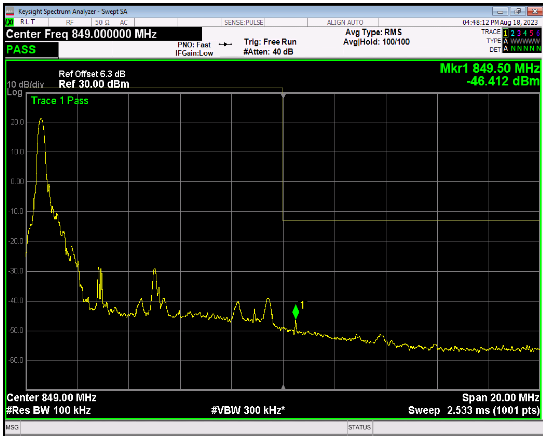
Band5 16QAM BW=10MHz Channel=20600 RB Size=1 Position=#Max
