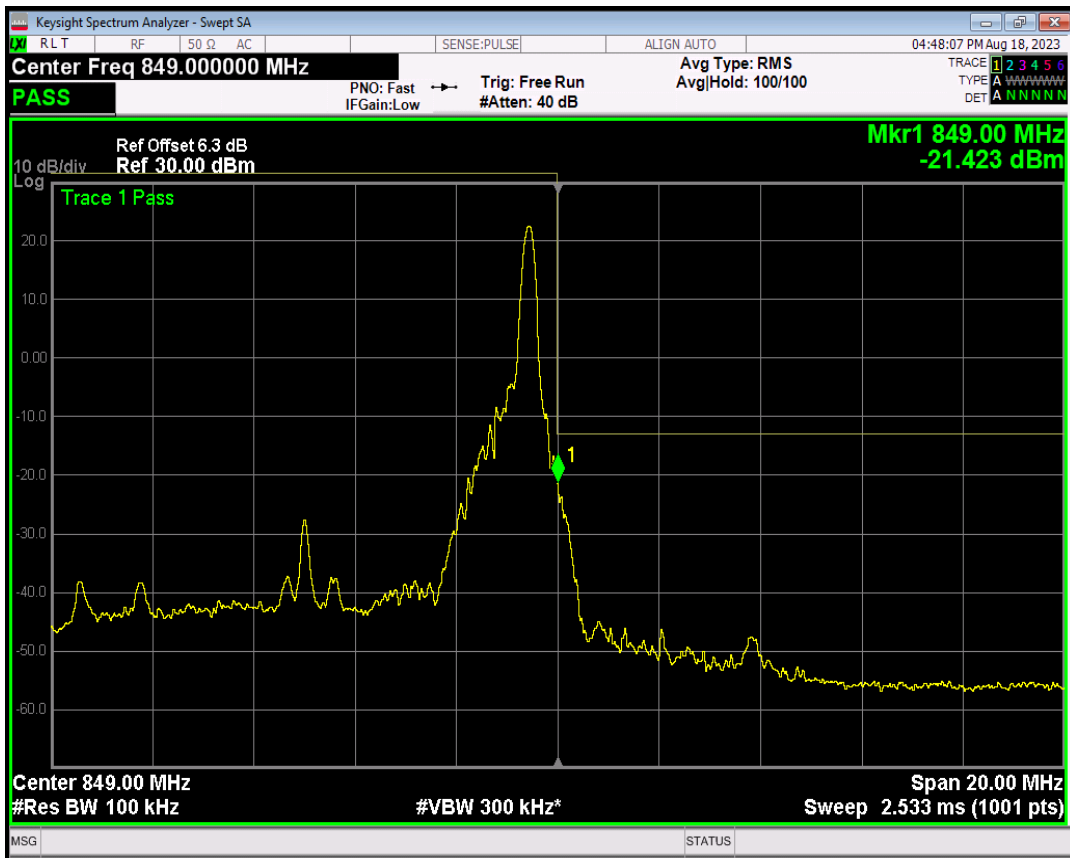
Band5 QPSK BW=10MHz Channel=20600 RB Size=50 Position=#0
