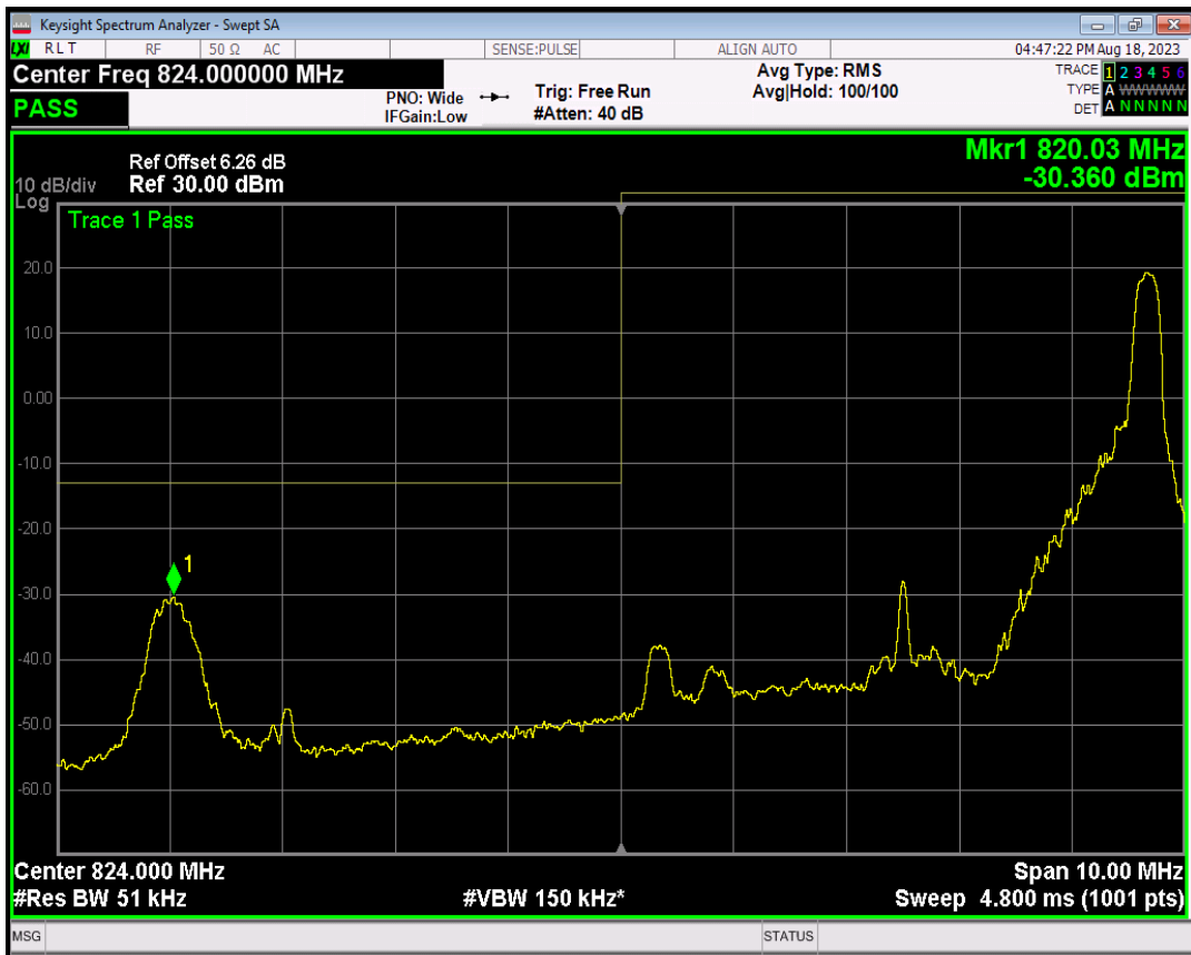
Band5 QPSK BW=5MHz Channel=20425 RB Size=25 Position=#0
