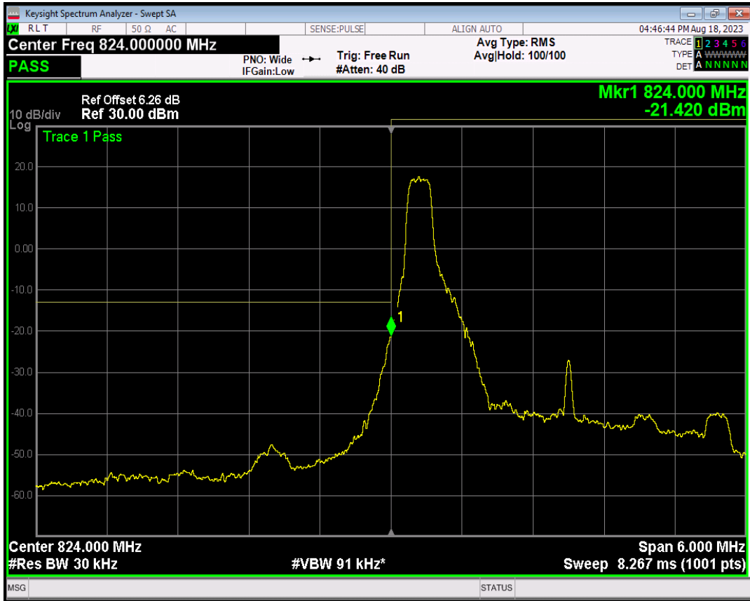
Band5 QPSK BW=3MHz Channel=20415 RB Size=1 Position=#Max
