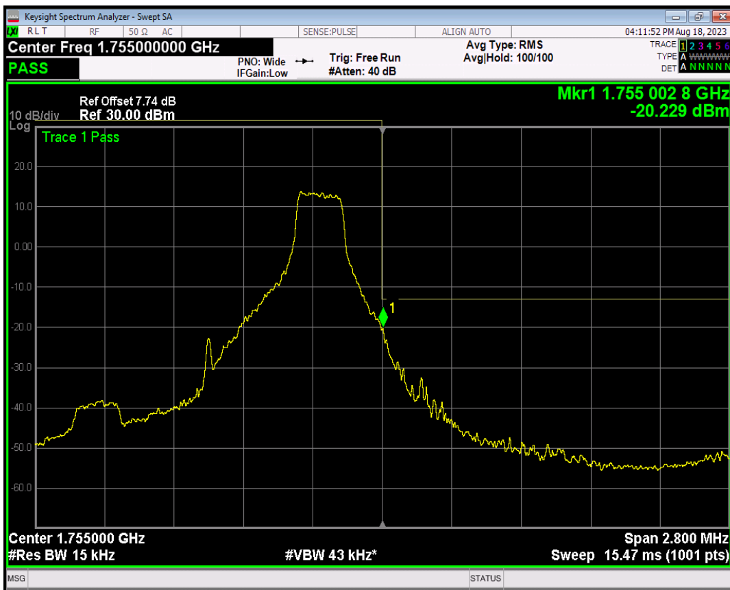
Band4 16QAM BW=1.4MHz Channel=20393 RB Size=6 Position=#0
