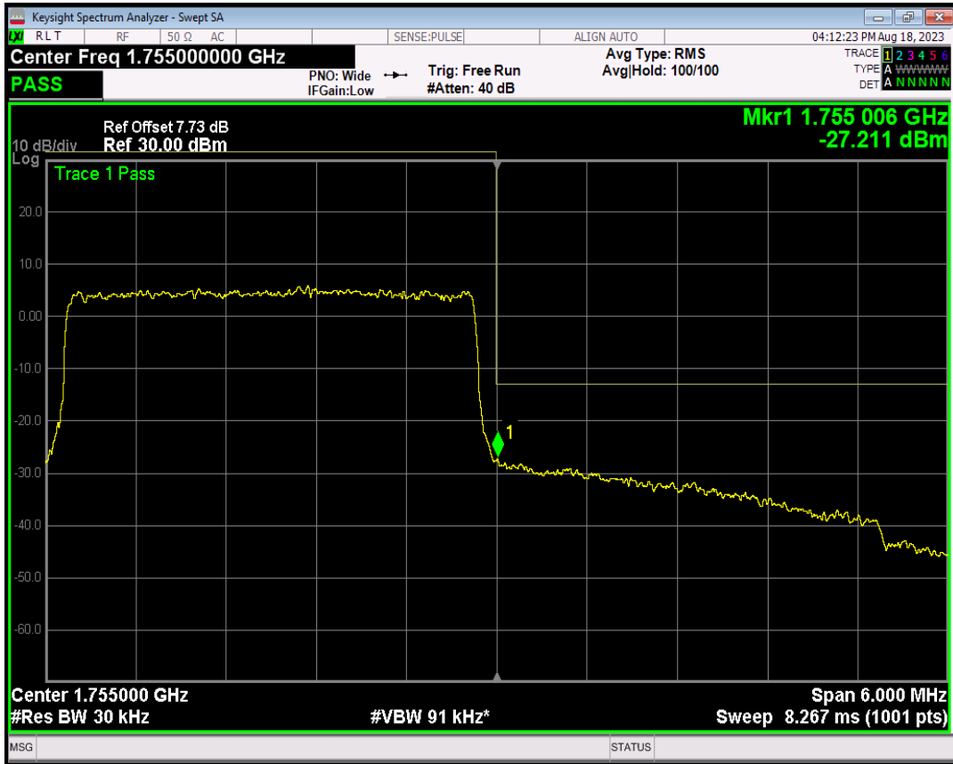
Band4 16QAM BW=3MHz Channel=20385 RB Size=1 Position=#0
