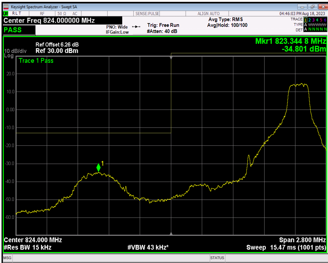
Band5 QPSK BW=1.4MHz Channel=20407 RB Size=6 Position=#0
