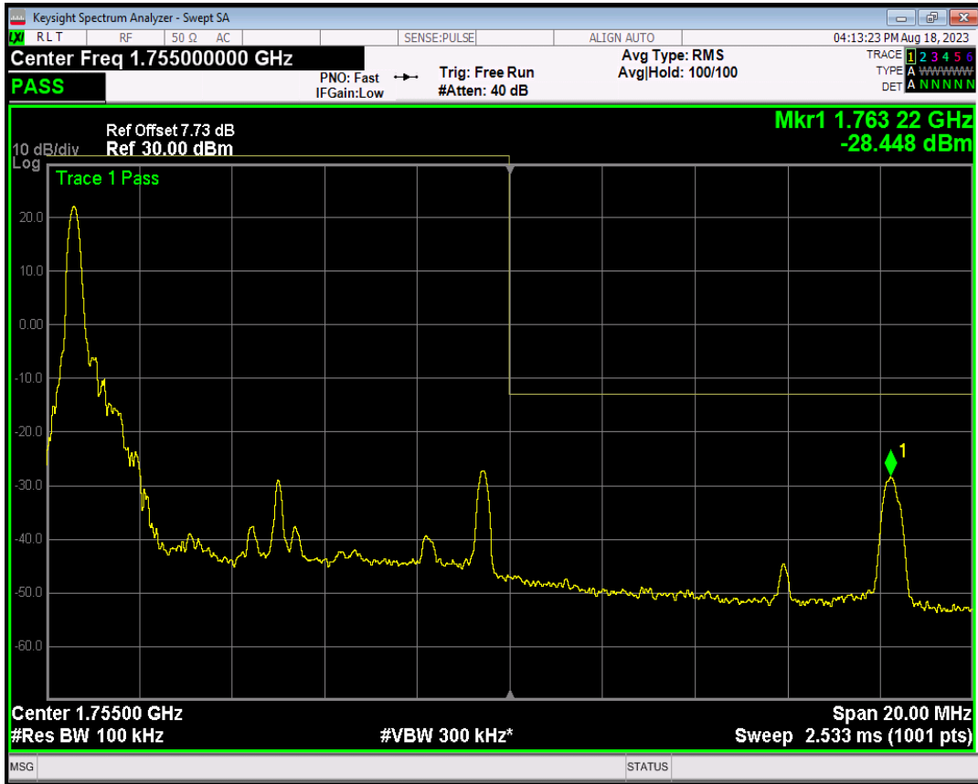
Band4 QPSK BW=10MHz Channel=20350 RB Size=1 Position=#Max
