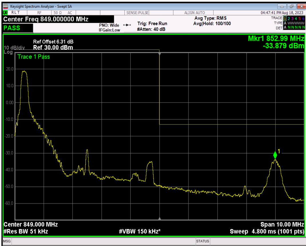
Band5 16QAM BW=5MHz Channel=20625 RB Size=1 Position=#Max
