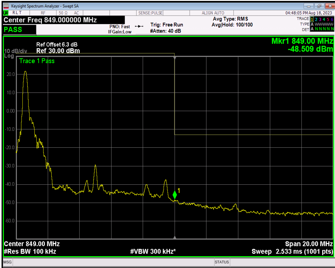
Band5 QPSK BW=10MHz Channel=20600 RB Size=1 Position=#Max
