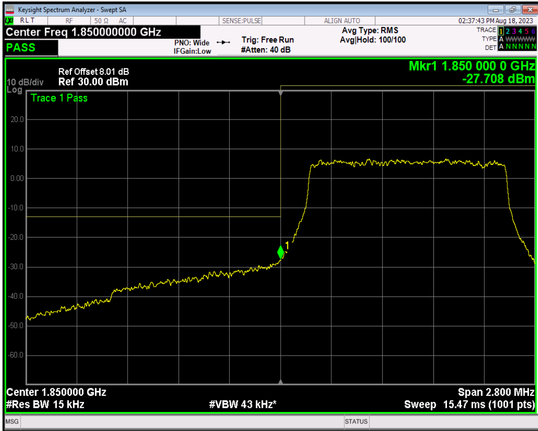
Band2 16QAM BW=1.4MHz Channel=18607 RB Size=1 Position=#0
