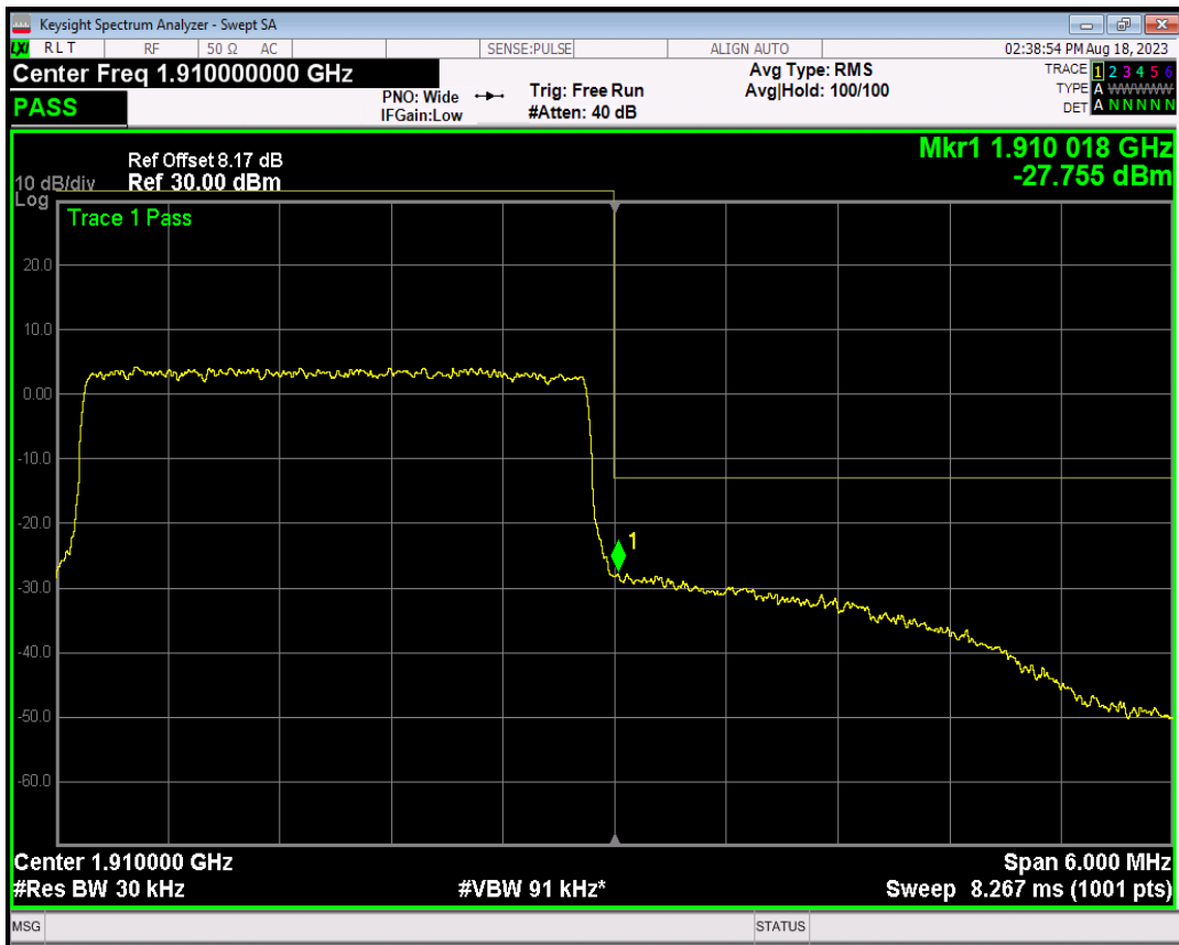
Band2 QPSK BW=5MHz Channel=18625 RB Size=1 Position=#0
