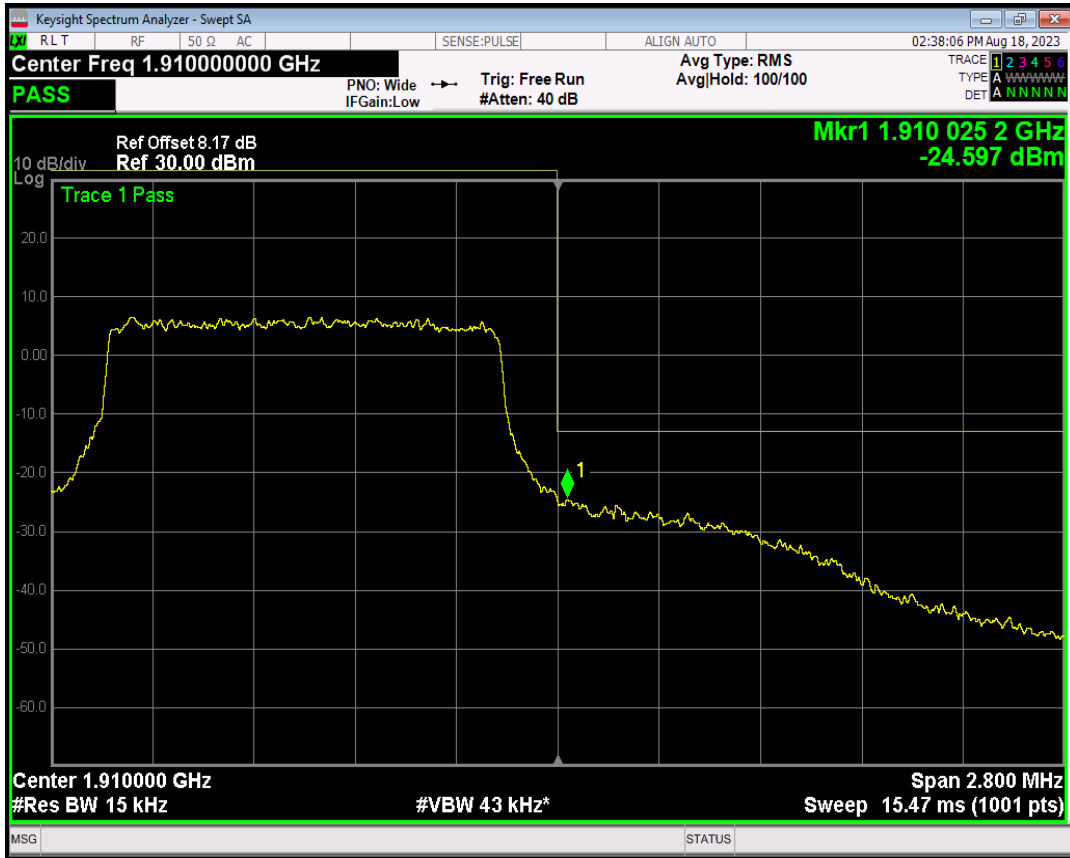
Band2 16QAM BW=1.4MHz Channel=19193 RB Size=1 Position=#0
