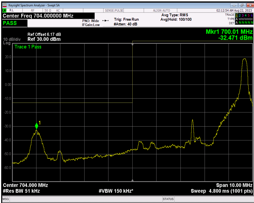
Band17 QPSK BW=5MHz Channel=23755 RB Size=25 Position=#0
