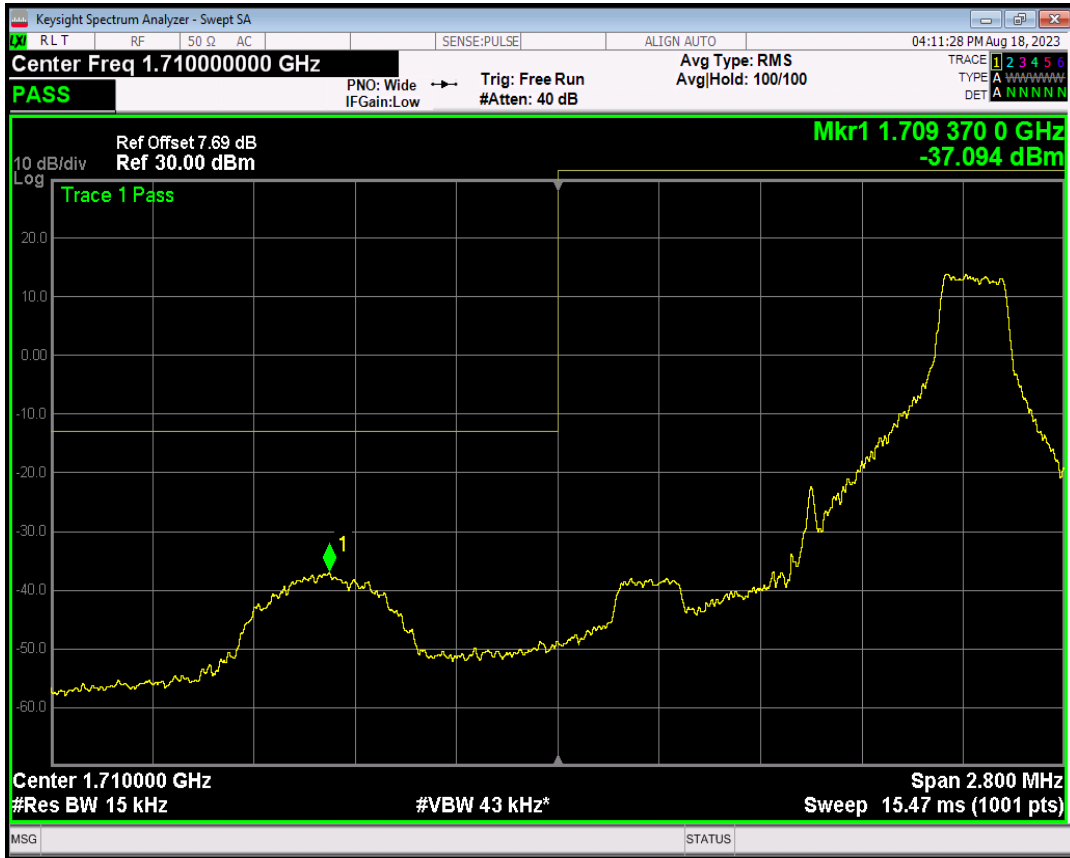
Band4 16QAM BW=1.4MHz Channel=19957 RB Size=6 Position=#0
