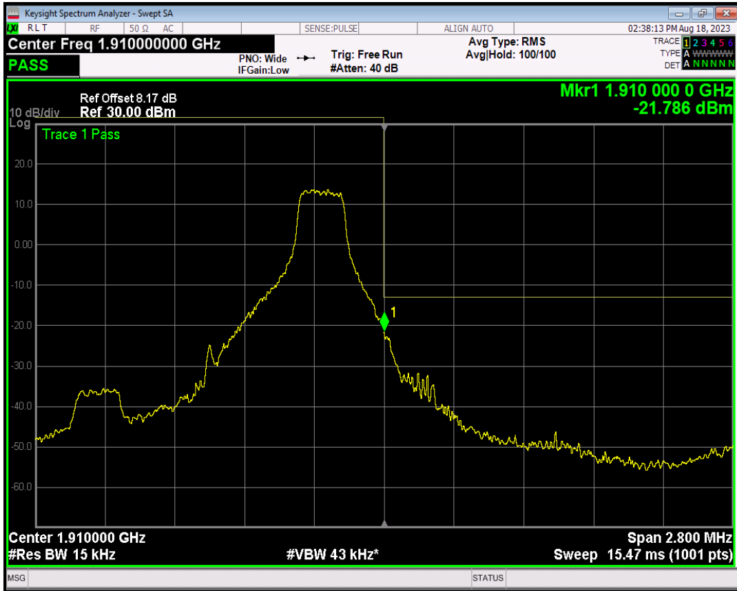
Band2 16QAM BW=1.4MHz Channel=19193 RB Size=6 Position=#0
