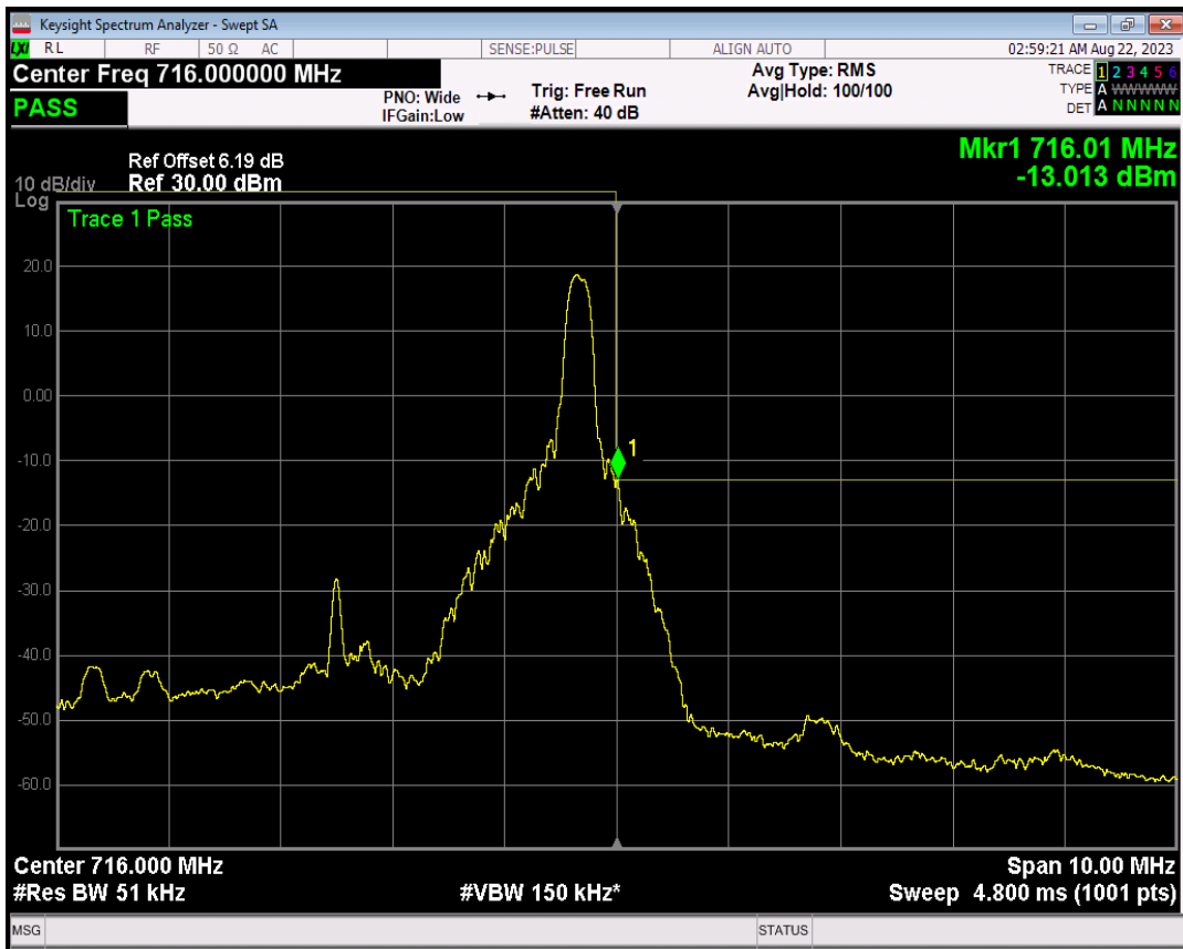
Band17 QPSK BW=5MHz Channel=23825 RB Size=25 Position=#0
