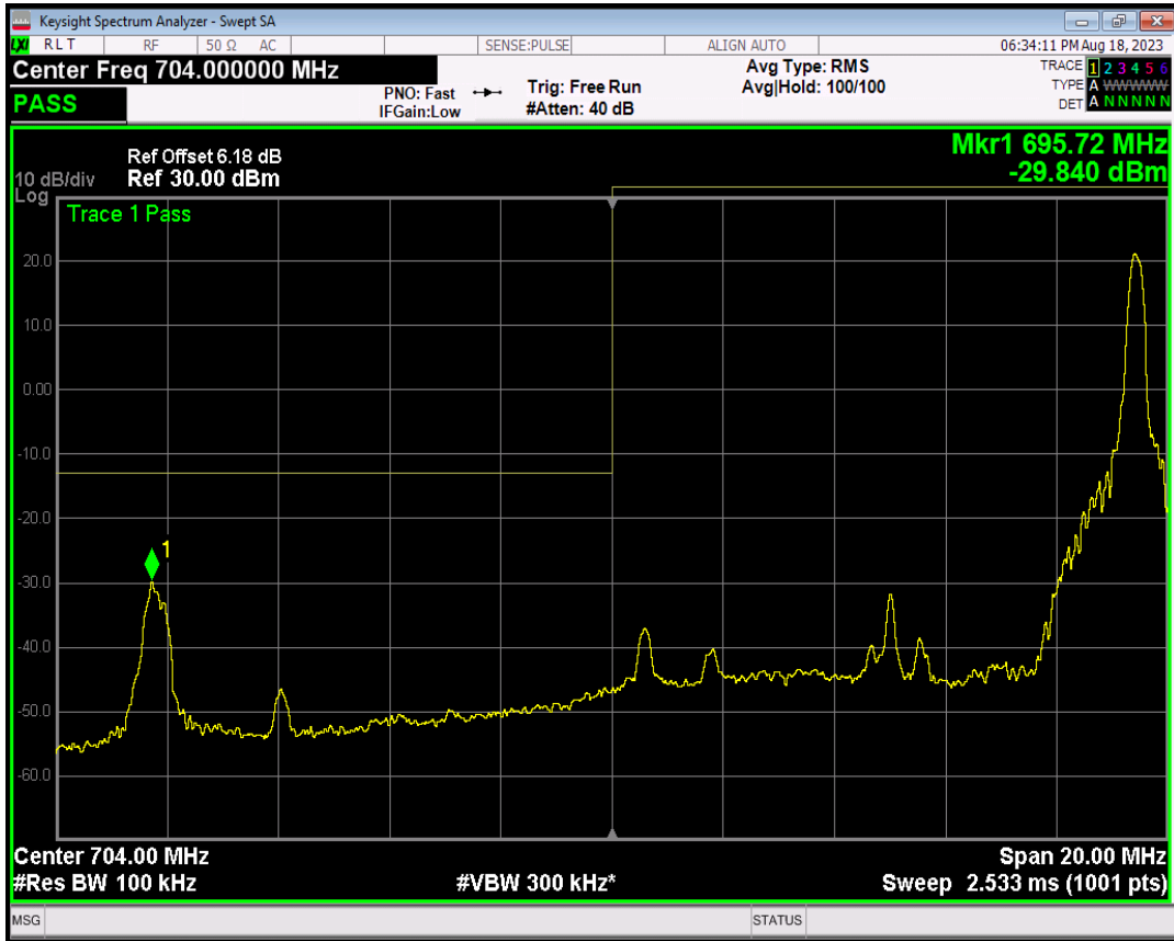
Band17 16QAM BW=10MHz Channel=23780 RB Size=50 Position=#0
