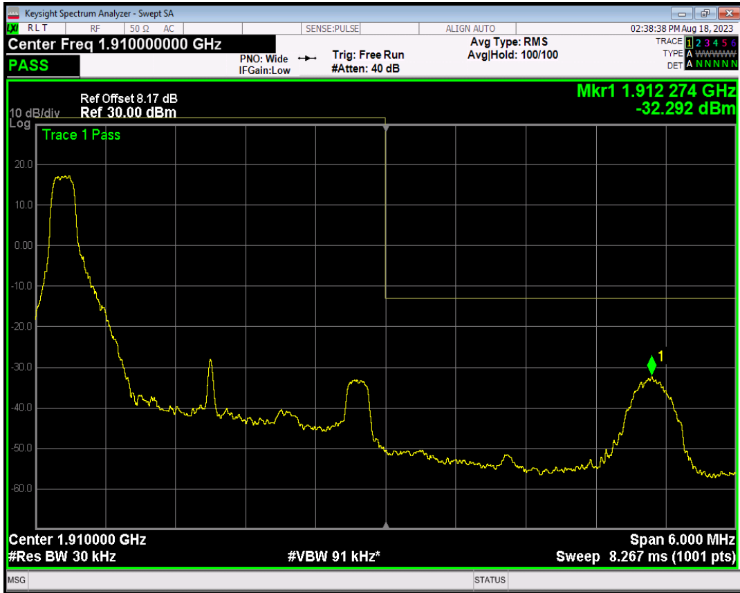
Band2 QPSK BW=3MHz Channel=19185 RB Size=1 Position=#Max
