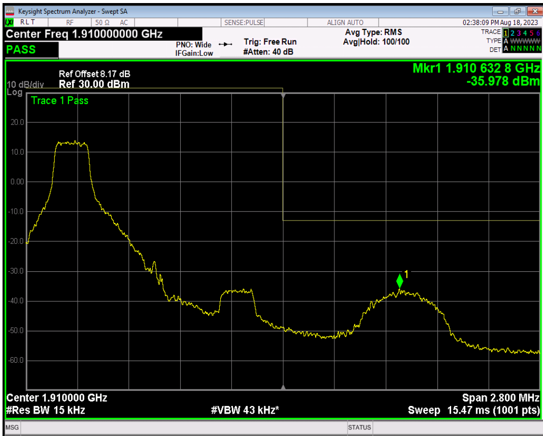
Band2 16QAM BW=1.4MHz Channel=19193 RB Size=1 Position=#Max
