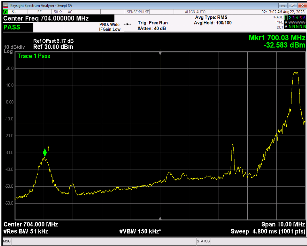
Band17 16QAM BW=5MHz Channel=23755 RB Size=25 Position=#0
