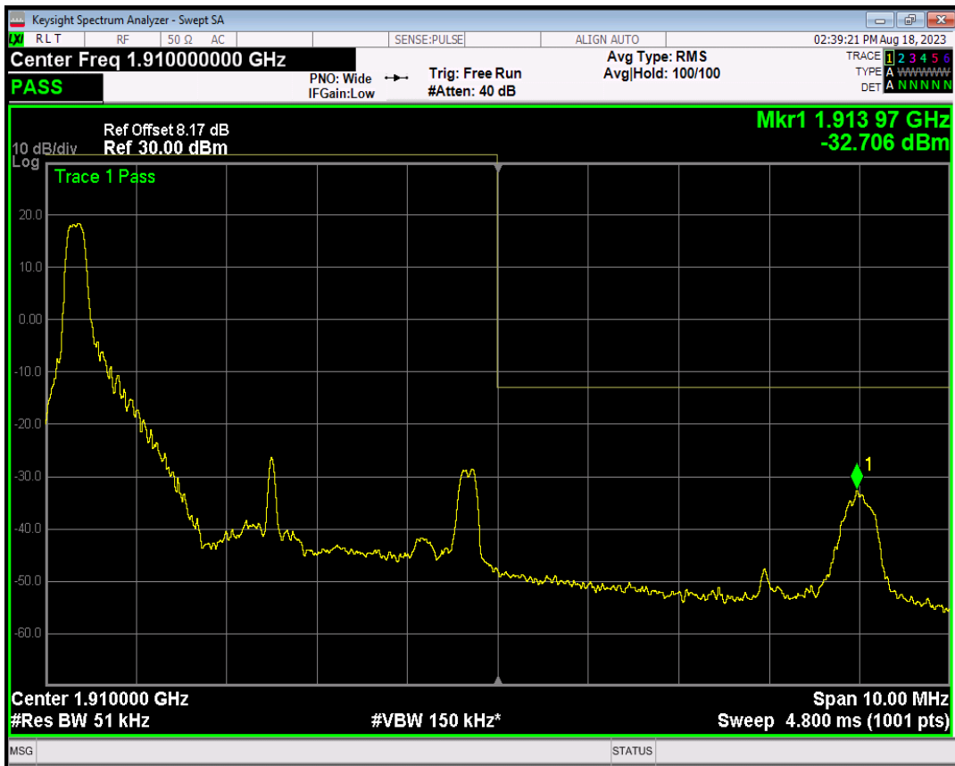
Band2 16QAM BW=5MHz Channel=19175 RB Size=1 Position=#Max
