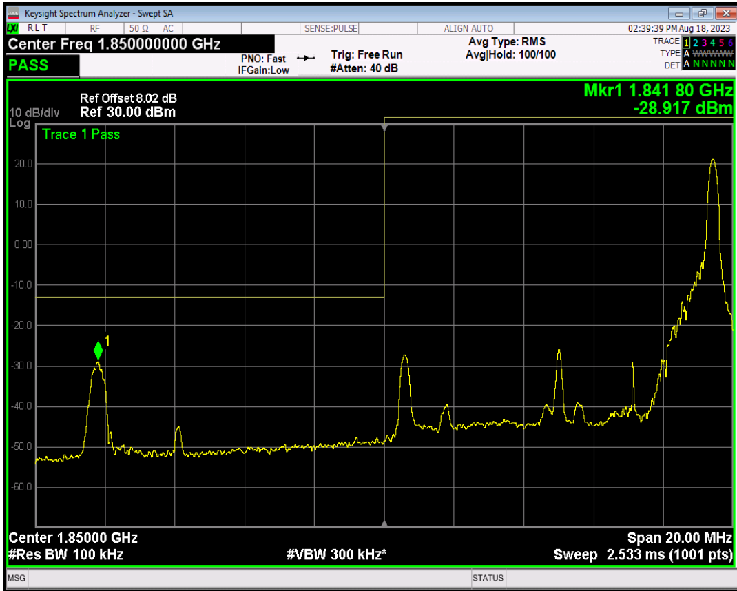
Band2 16QAM BW=10MHz Channel=18650 RB Size=50 Position=#0
