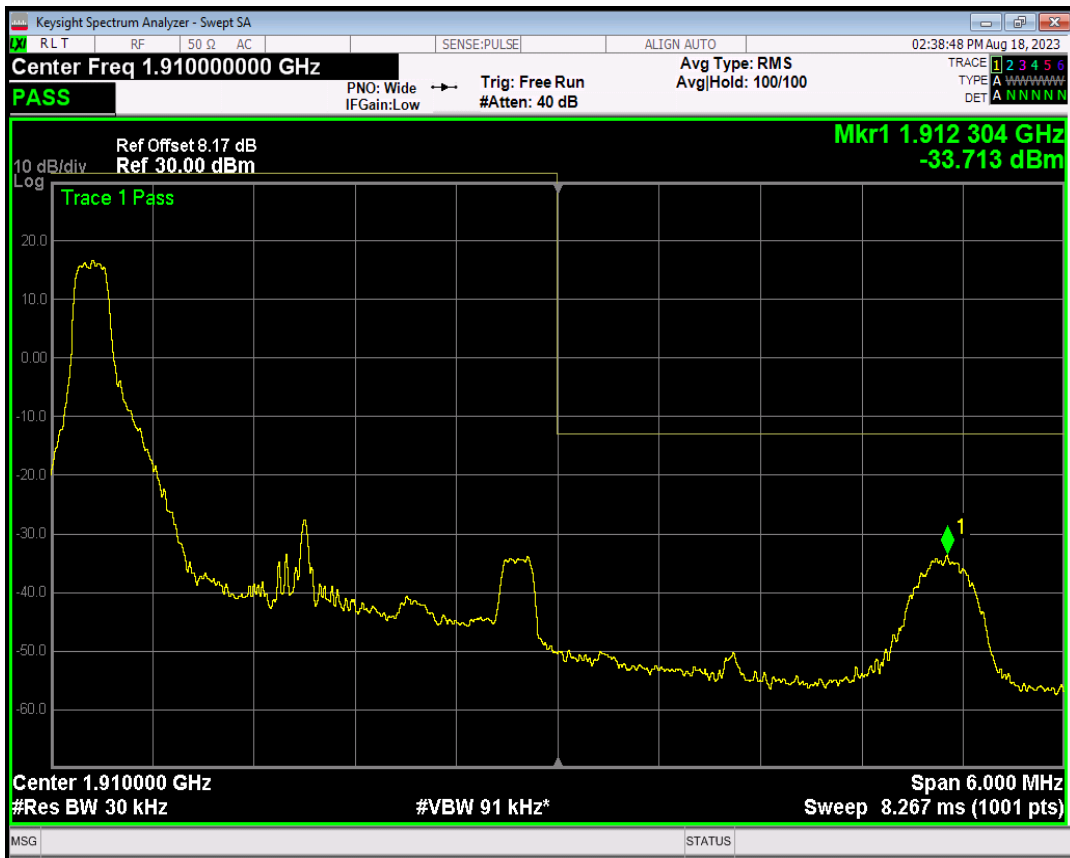
Band2 16QAM BW=3MHz Channel=19185 RB Size=1 Position=#Max
