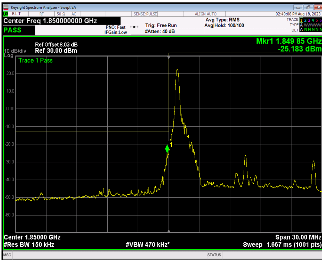
Band2 16QAM BW=15MHz Channel=18675 RB Size=1 Position=#Max
