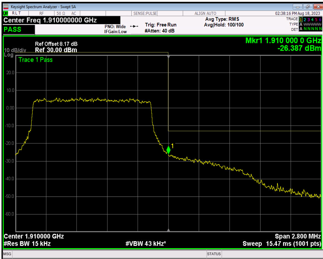
Band2 QPSK BW=3MHz Channel=18615 RB Size=1 Position=#Max
