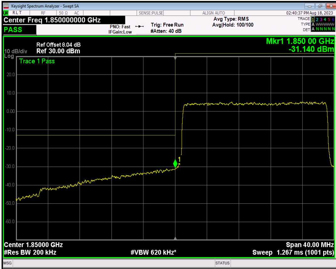
Band2 16QAM BW=20MHz Channel=18700 RB Size=1 Position=#0
