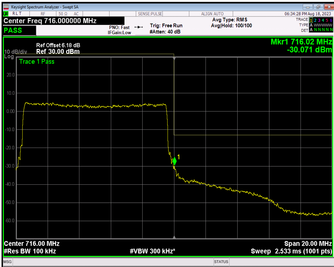
Band2 QPSK BW=1.4MHz Channel=18607 RB Size=1 Position=#Max
