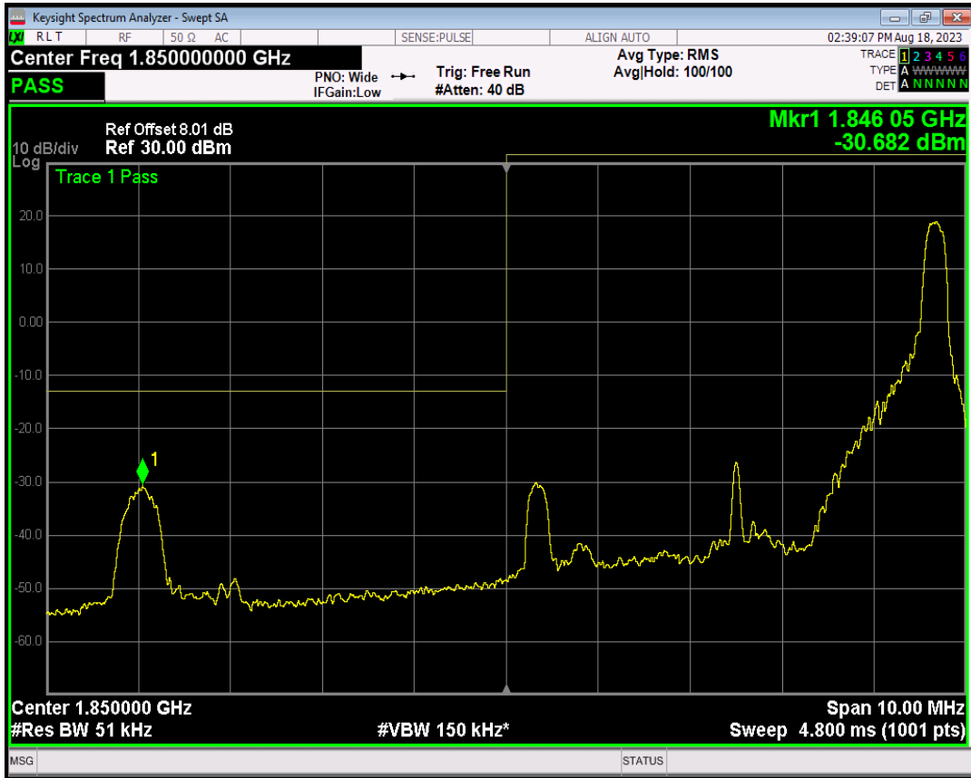
Band2 16QAM BW=5MHz Channel=18625 RB Size=25 Position=#0
