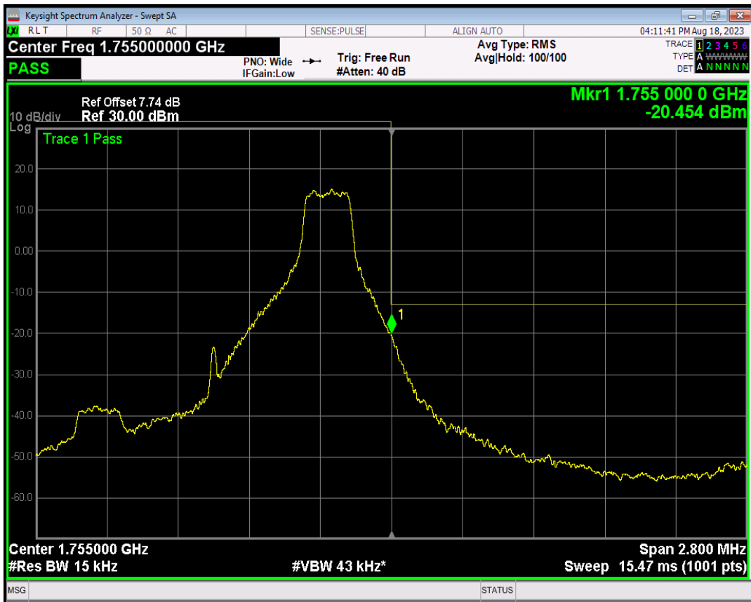
Band4 QPSK BW=1.4MHz Channel=20393 RB Size=6 Position=#0
