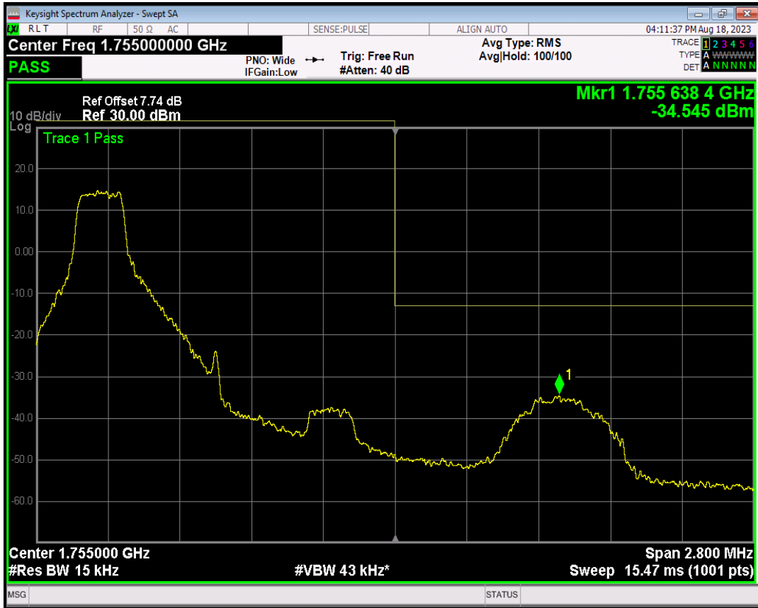
Band4 QPSK BW=1.4MHz Channel=20393 RB Size=1 Position=#Max
