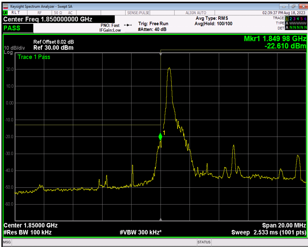
Band2 16QAM BW=10MHz Channel=18650 RB Size=1 Position=#Max
