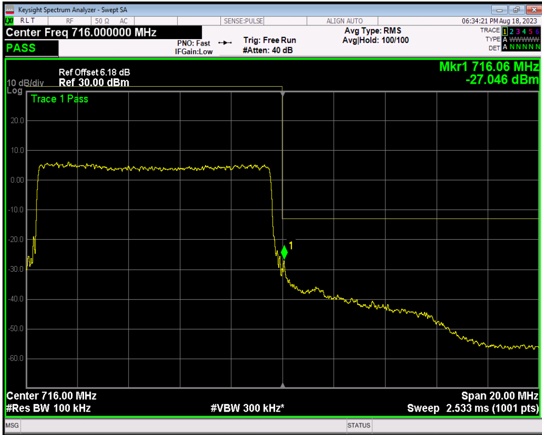
Band17 16QAM BW=10MHz Channel=23800 RB Size=1 Position=#0
