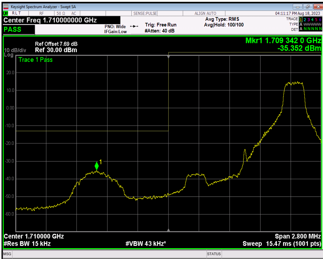
Band4 16QAM BW=1.4MHz Channel=19957 RB Size=1 Position=#0
