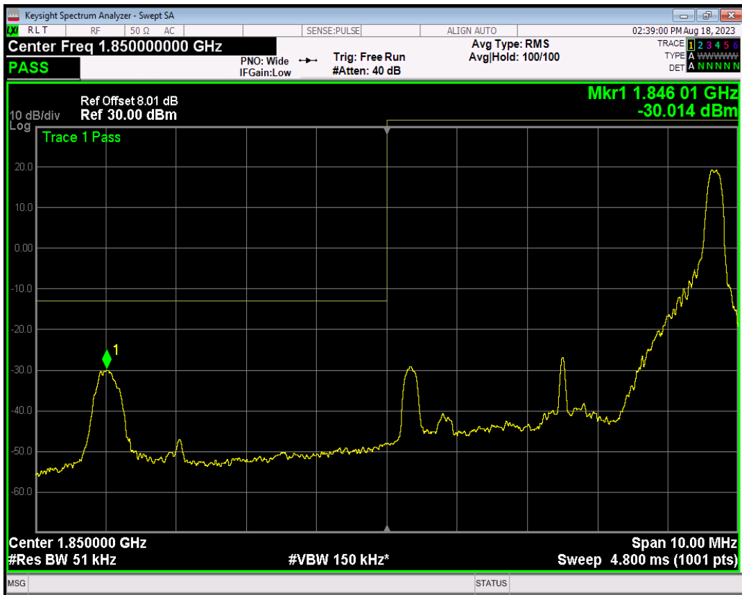
Band2 QPSK BW=5MHz Channel=18625 RB Size=25 Position=#0
