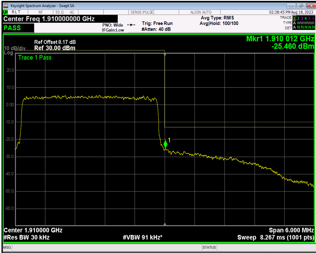
Band2 16QAM BW=3MHz Channel=19185 RB Size=1 Position=#0
