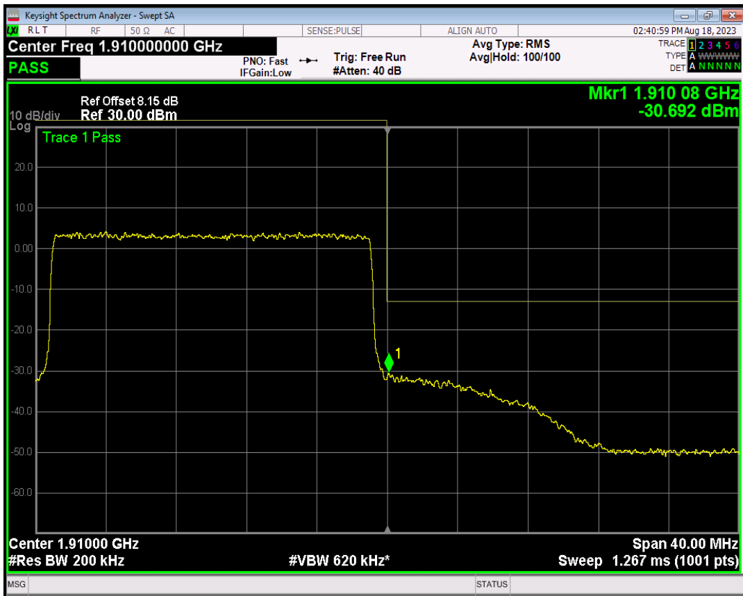
Band4 QPSK BW=1.4MHz Channel=19957 RB Size=1 Position=#0
