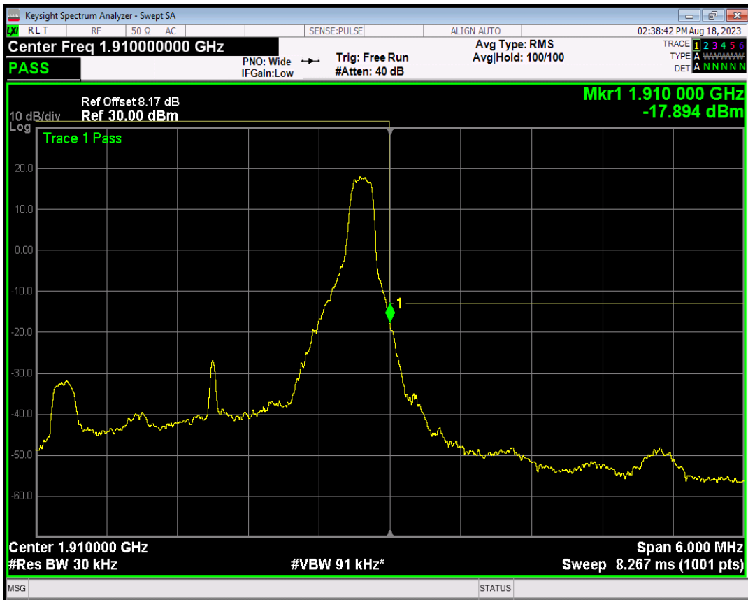
Band2 QPSK BW=3MHz Channel=19185 RB Size=15 Position=#0
