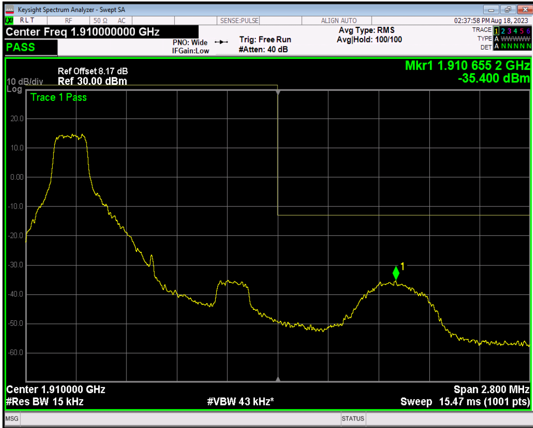
Band2 QPSK BW=1.4MHz Channel=19193 RB Size=1 Position=#Max
