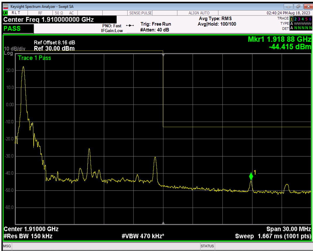
Band2 16QAM BW=15MHz Channel=19125 RB Size=1 Position=#Max
