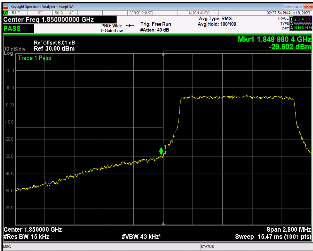
Band2 QPSK BW=1.4MHz Channel=19193 RB Size=1 Position=#0
