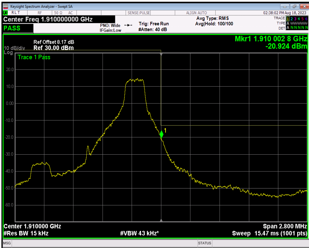
Band2 QPSK BW=1.4MHz Channel=19193 RB Size=6 Position=#0
