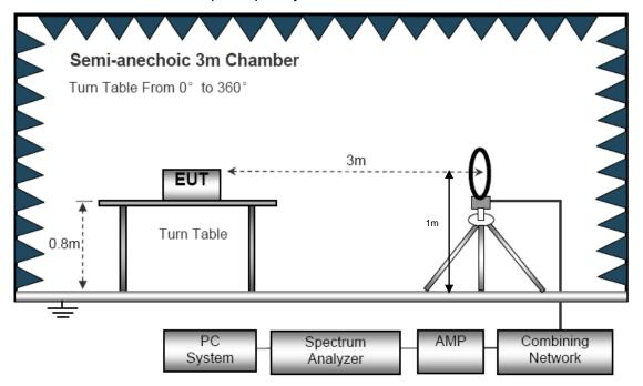
(B) Radiated Emission Test-Up Frequency 30MHz~1GHz
