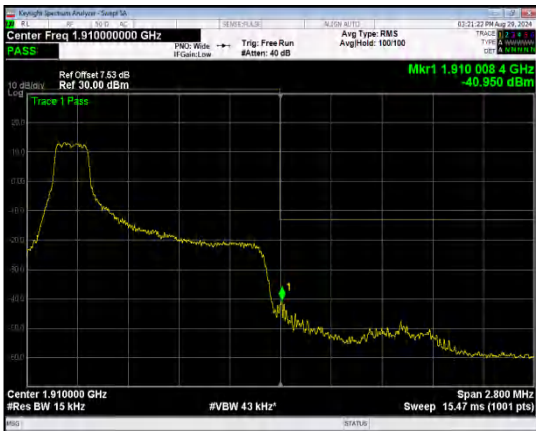
Band2 QPSK BW=1.4MHz Channel=19193 RB Size=6 Position=#0
