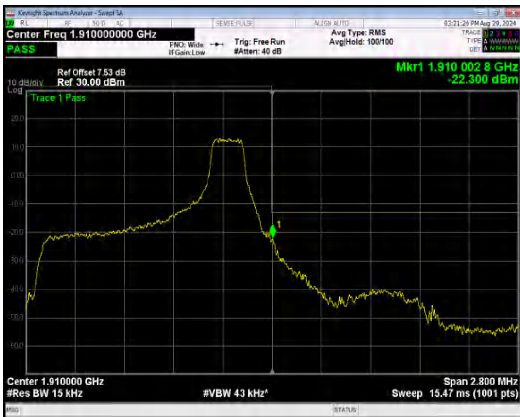
Band2 16QAM BW=1.4MHz Channel=19193 RB Size=6 Position=#0
