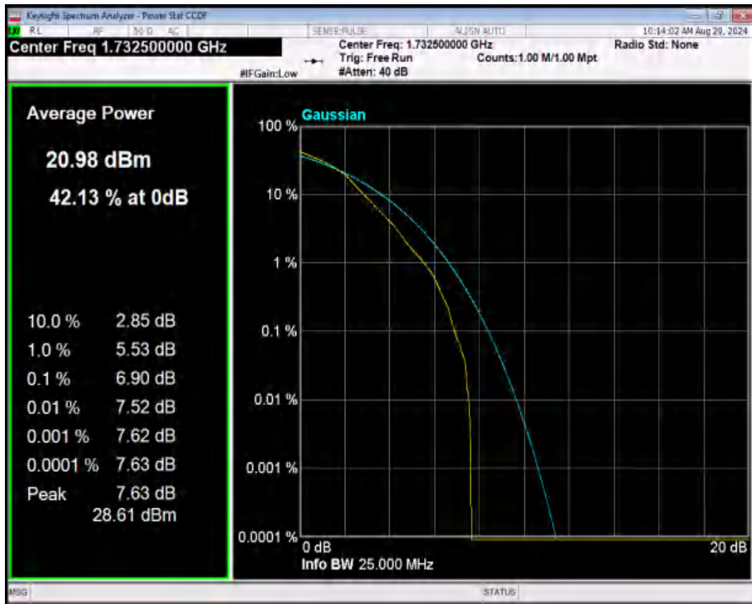
Band4 QPSK BW=10MHz Channel=20175 RB Size=1 Position=#0
