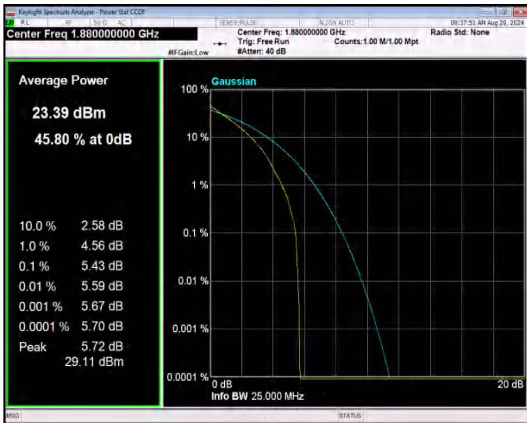
Band2 16QAM BW=3MHz Channel=18900 RB Size=1 Position=#0
