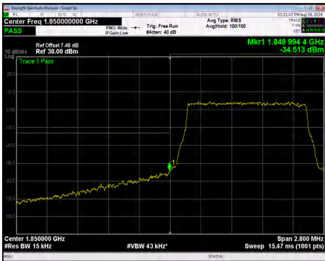
Band2 QPSK BW=1.4MHz Channel=19193 RB Size=1 Position=#0
