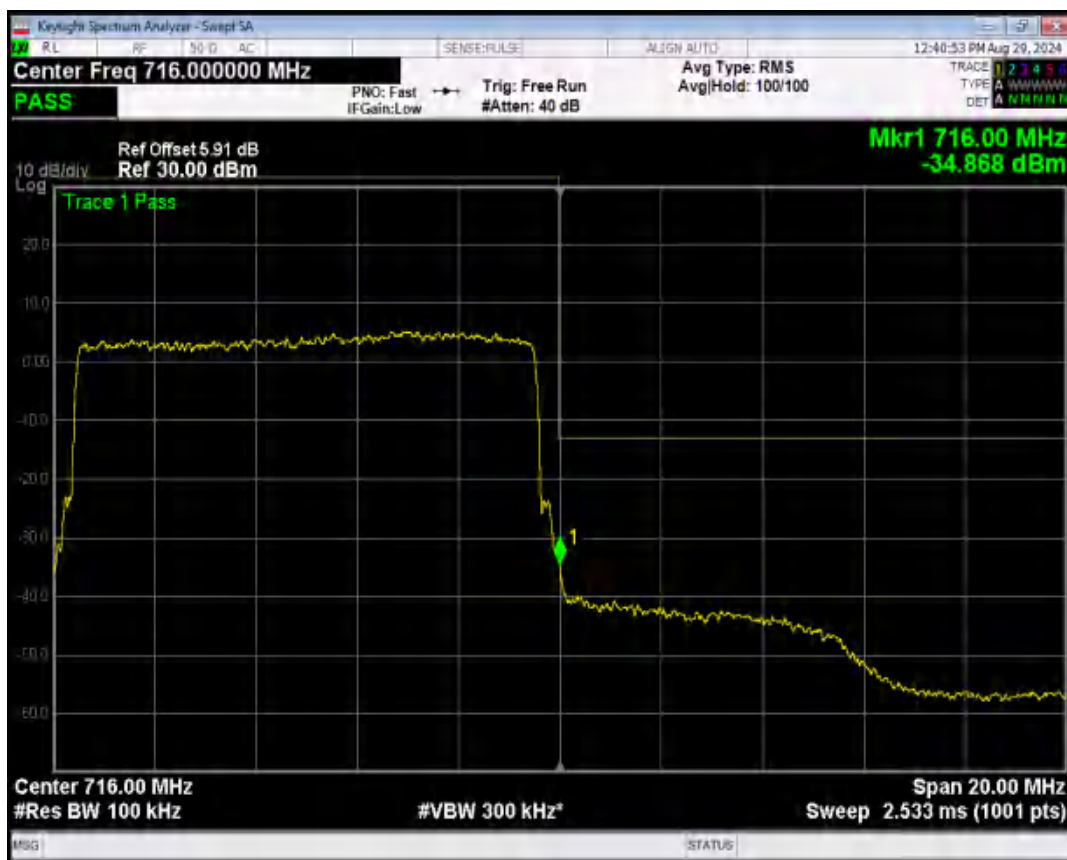
Band17 16QAM BW=10MHz Channel=23800 RB Size=1 Position=#0
