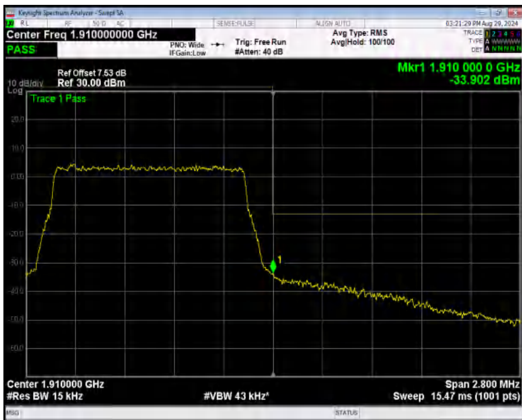
Band2 QPSK BW=3MHz Channel=18615 RB Size=1 Position=#0
