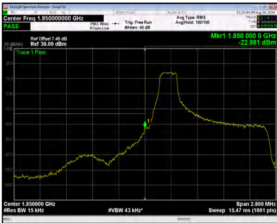
Band2 QPSK BW=1.4MHz Channel=18607 RB Size=1 Position=#Max
