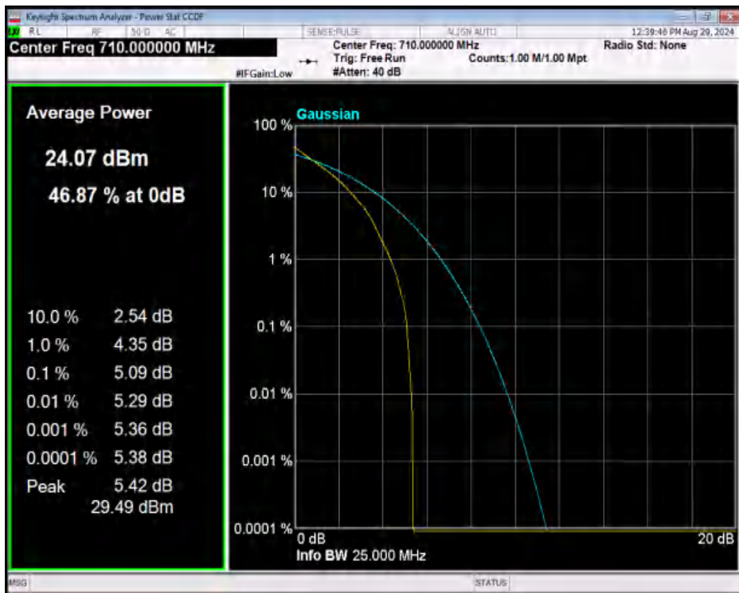
Band17 16QAM BW=10MHz Channel=23790 RB Size=1 Position=#0
