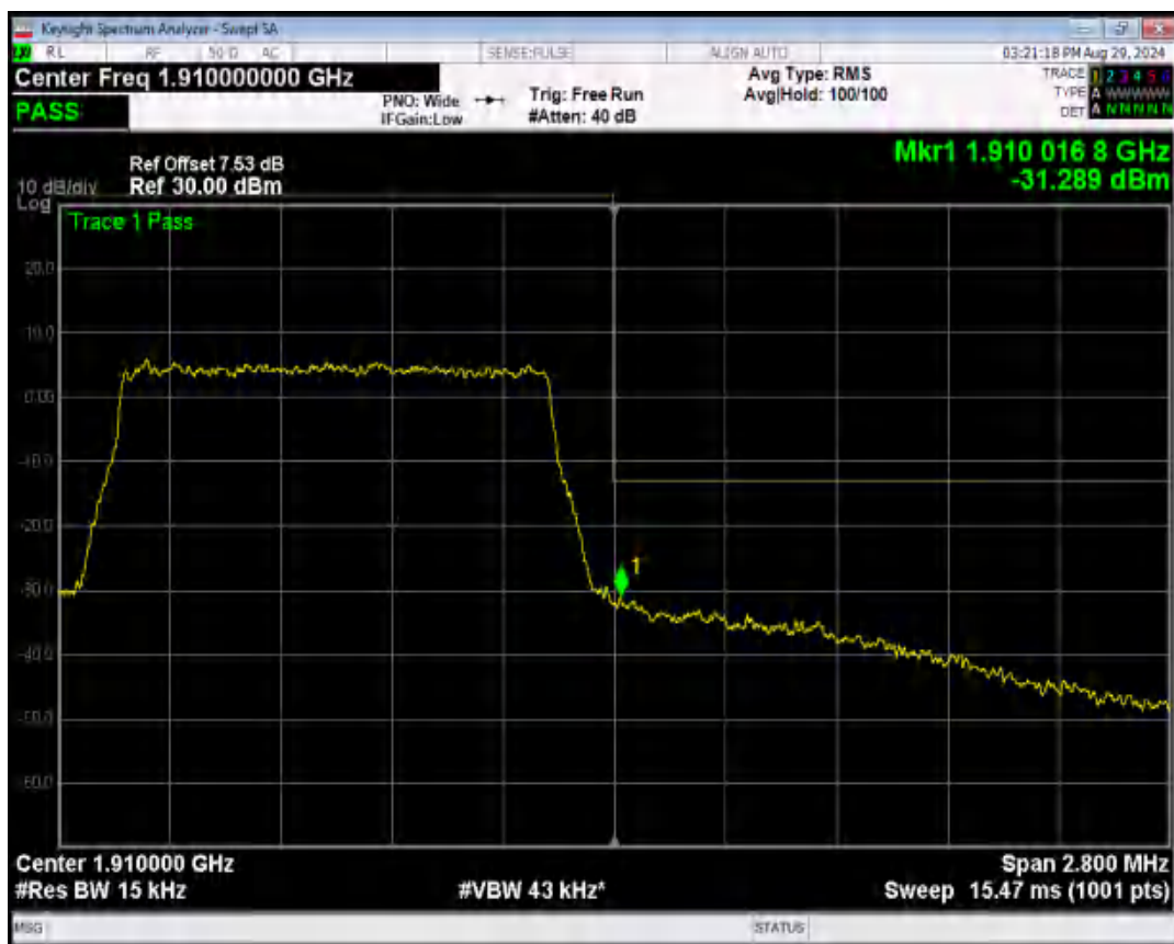
Band2 16QAM BW=1.4MHz Channel=19193 RB Size=1 Position=#Max
