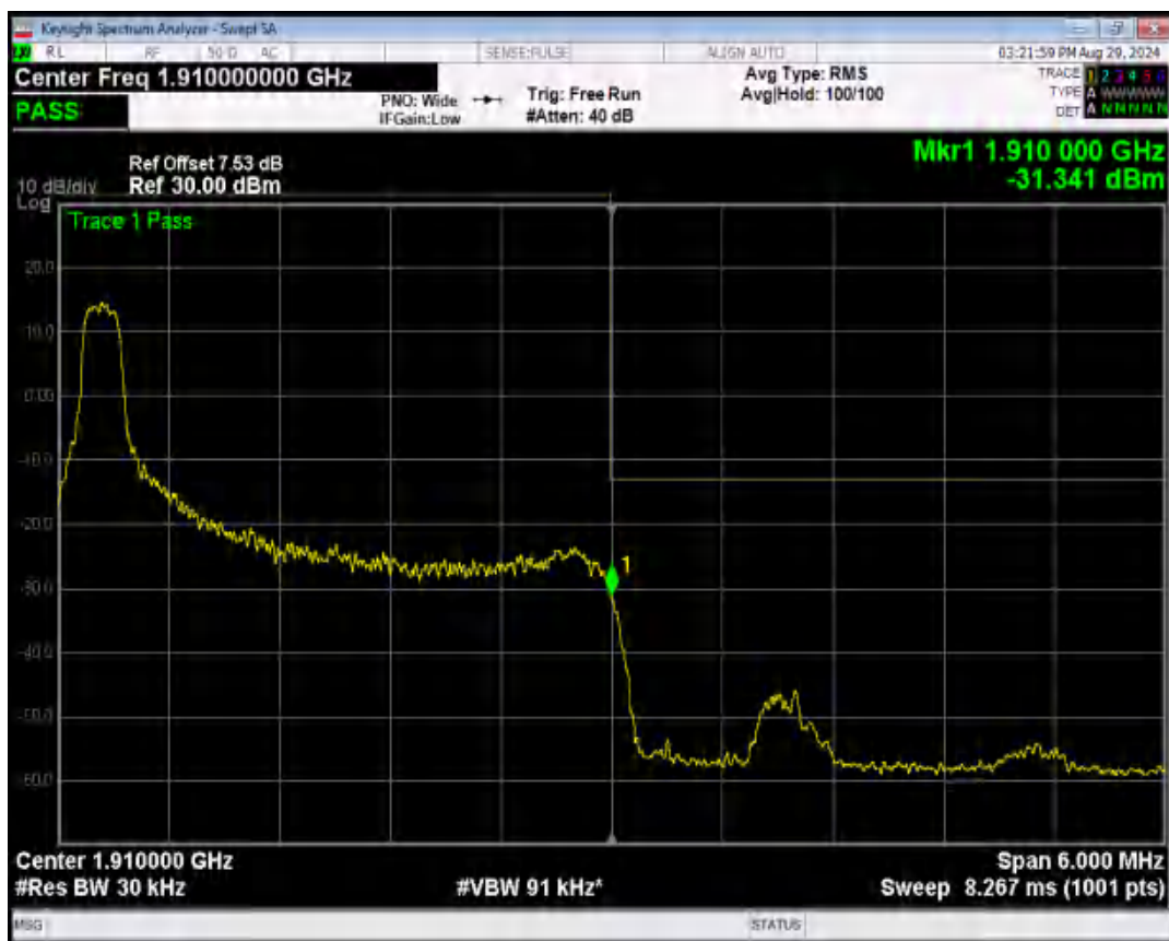
Band2 16QAM BW=3MHz Channel=19185 RB Size=1 Position=#Max
