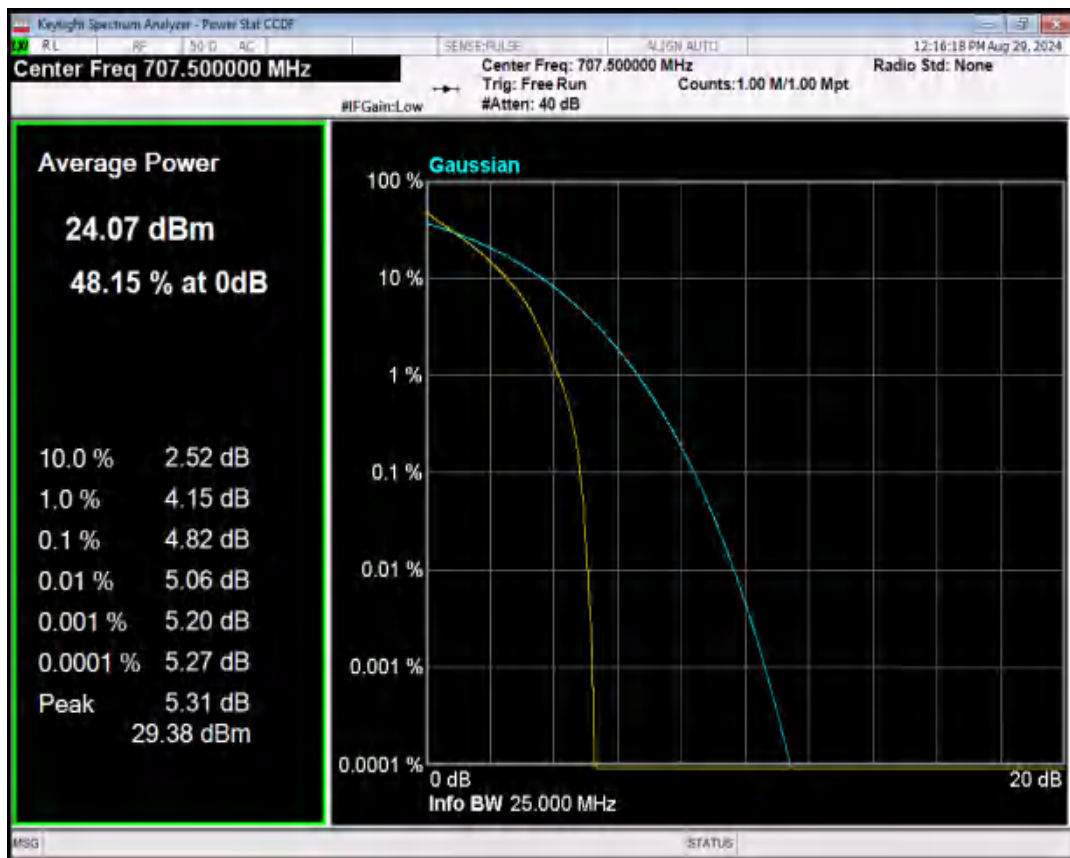
Band12 16QAM BW=5MHz Channel=23095 RB Size=1 Position=#0
