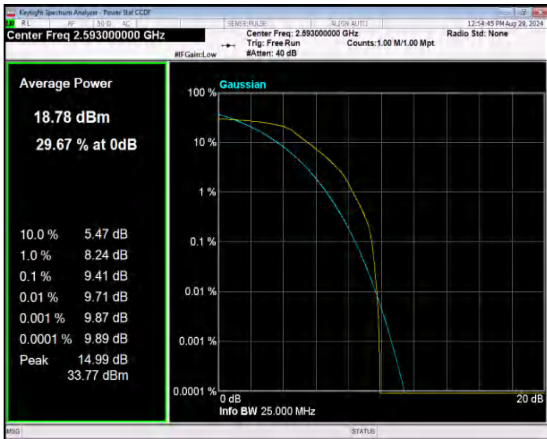
Band41 16QAM BW=10MHz Channel=40620 RB Size=1 Position=#0
