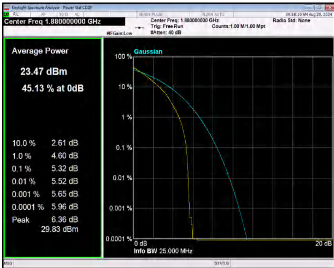
Band2 16QAM BW=20MHz Channel=18900 RB Size=1 Position=#0
