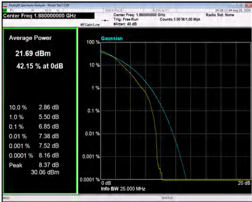
Band4 QPSK BW=1.4MHz Channel=20175 RB Size=1 Position=#0
