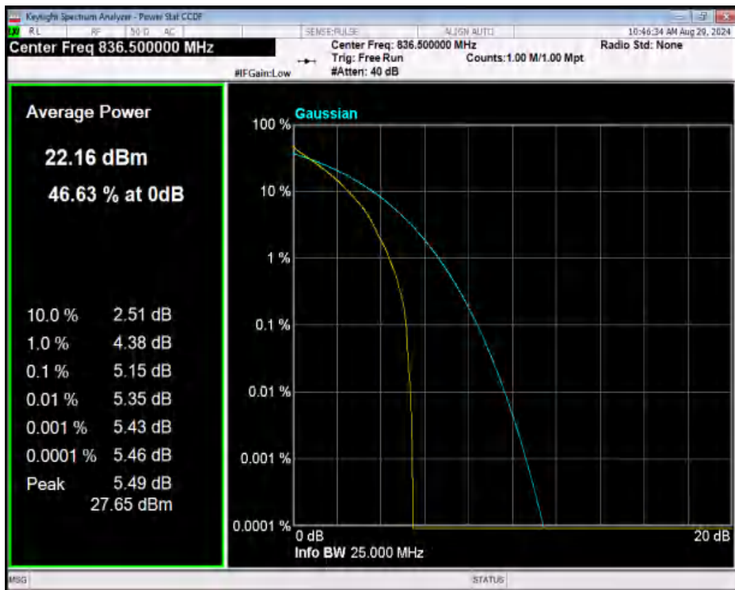
Band5 16QAM BW=3MHz Channel=20525 RB Size=1 Position=#0
