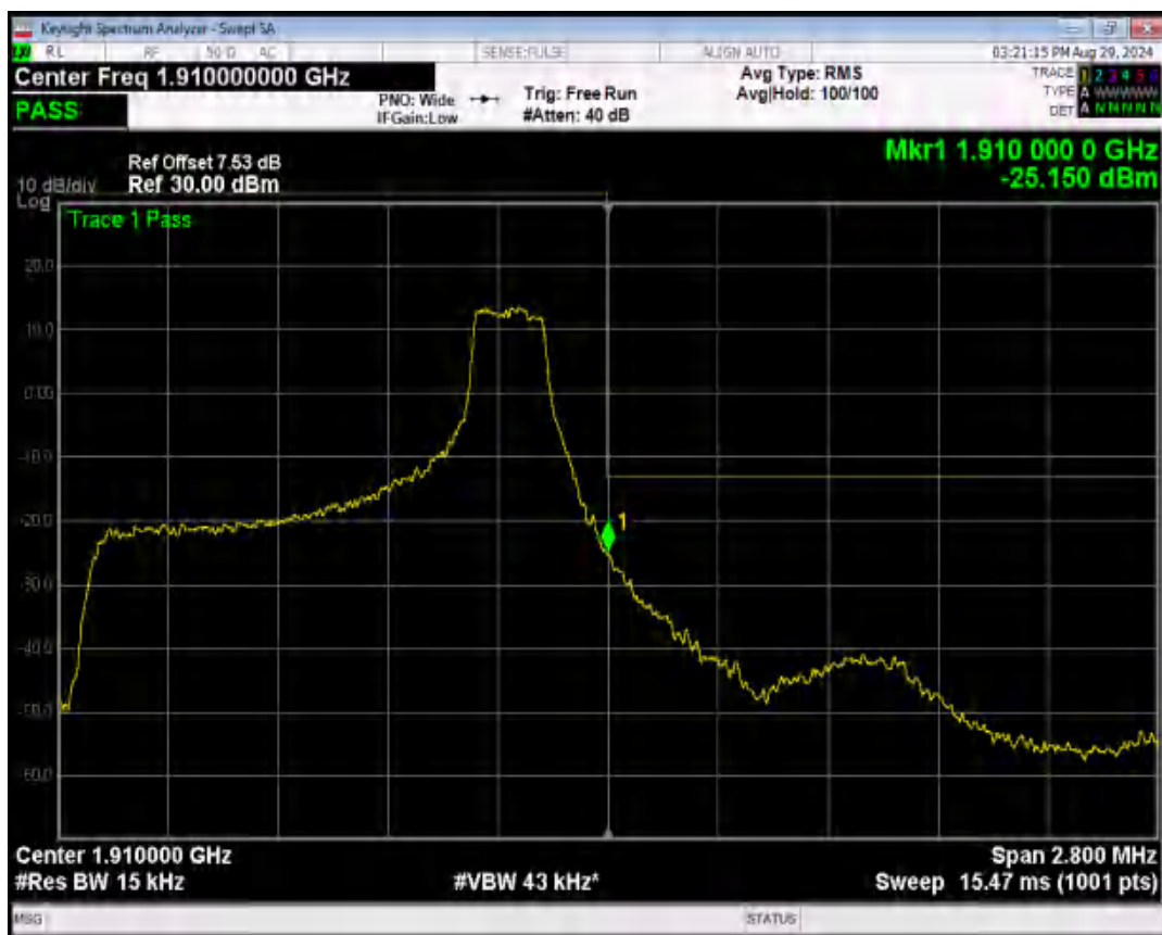
Band2 16QAM BW=1.4MHz Channel=19193 RB Size=1 Position=#0
