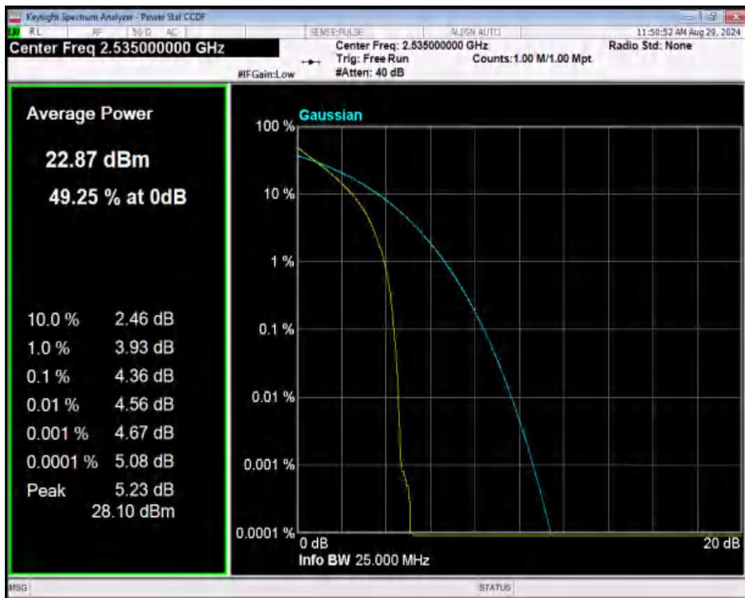
Band7 16QAM BW=15MHz Channel=21100 RB Size=1 Position=#0
