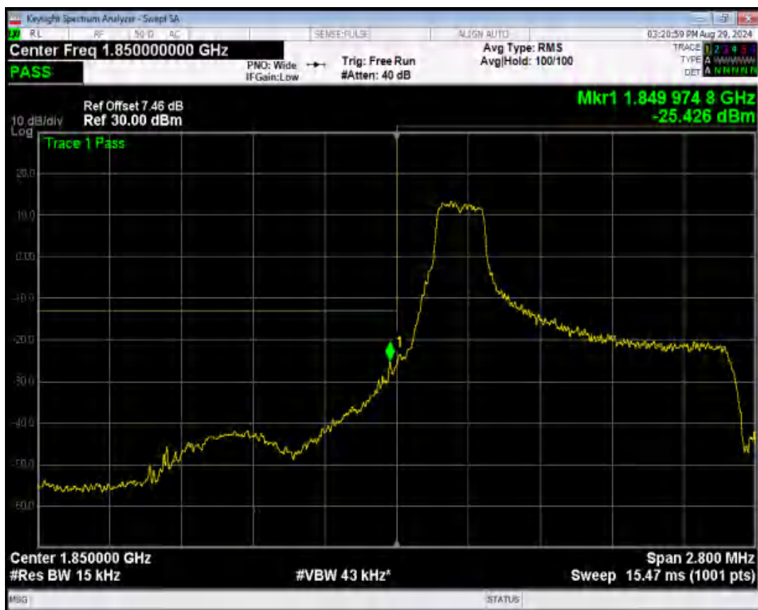
Band2 16QAM BW=1.4MHz Channel=18607 RB Size=1 Position=#Max
