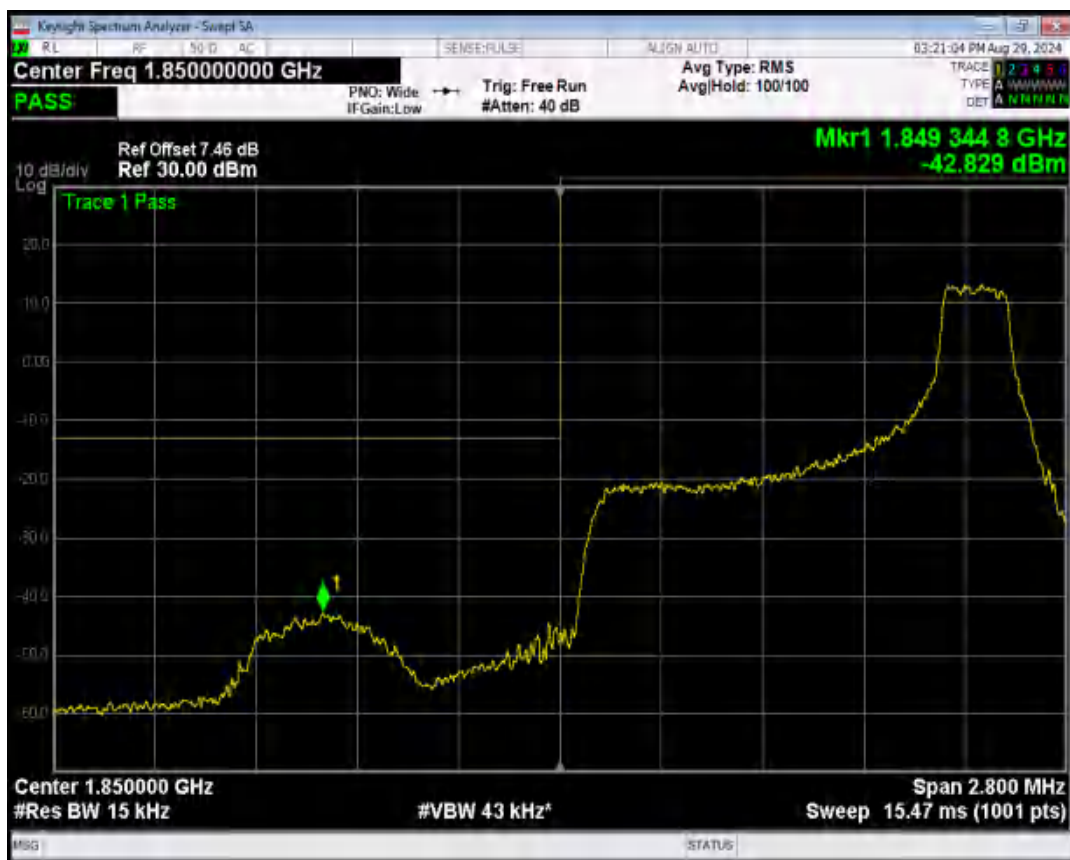
Band2 16QAM BW=1.4MHz Channel=18607 RB Size=6 Position=#0
