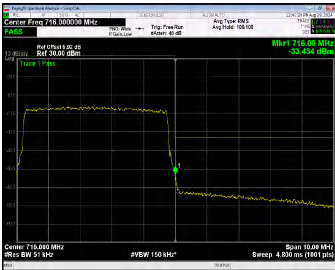
Band17 QPSK BW=10MHz Channel=23780 RB Size=1 Position=#Max
