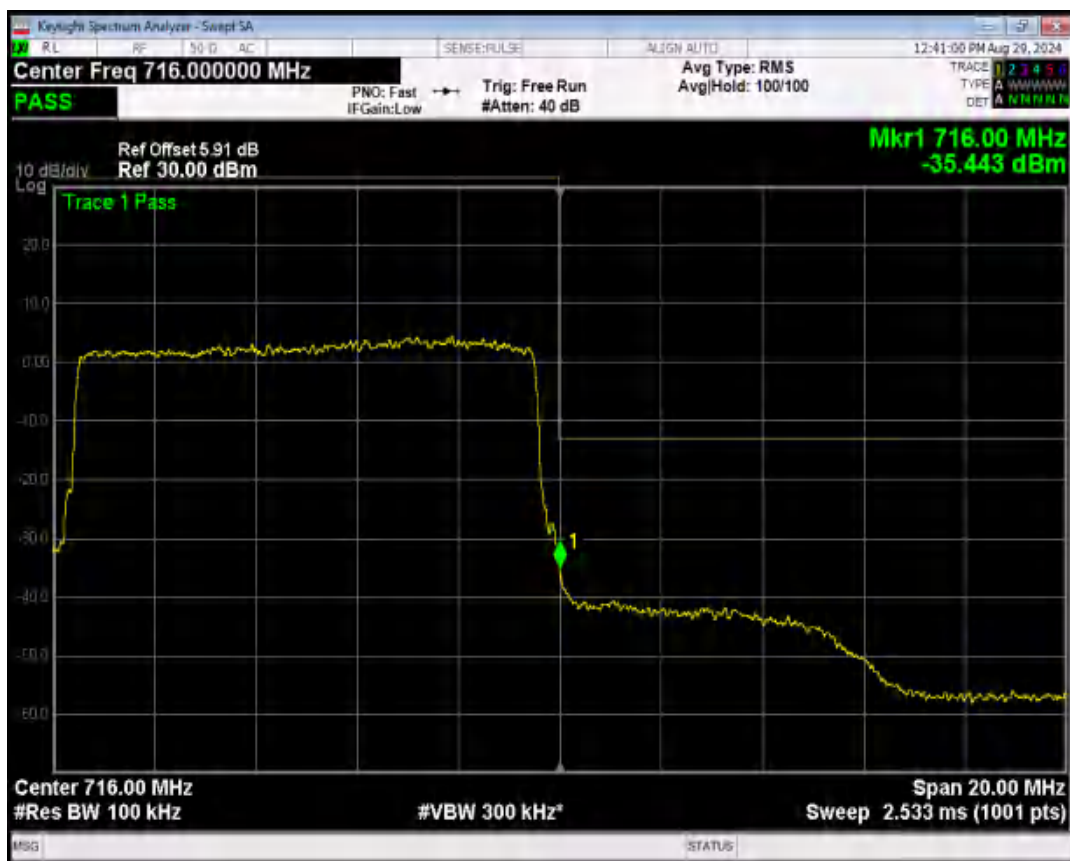
Band2 QPSK BW=1.4MHz Channel=18607 RB Size=1 Position=#0
