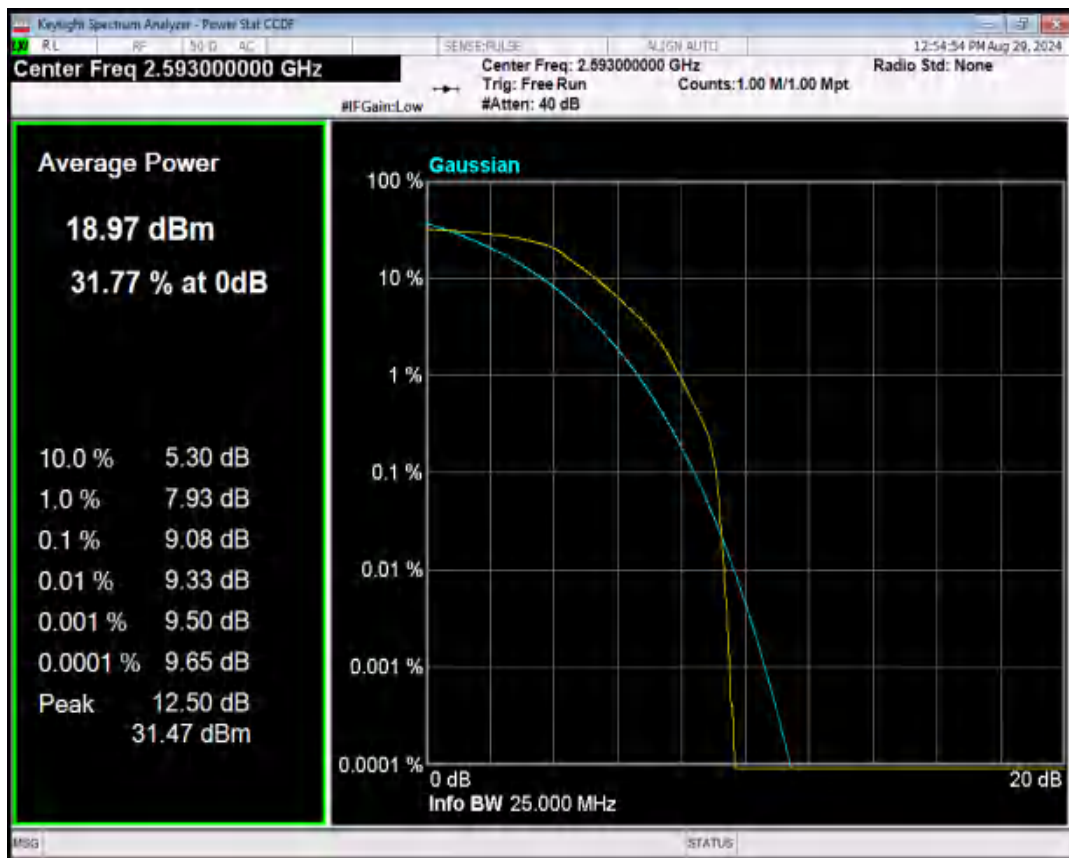
Band41 16QAM BW=20MHz Channel=40620 RB Size=1 Position=#0
