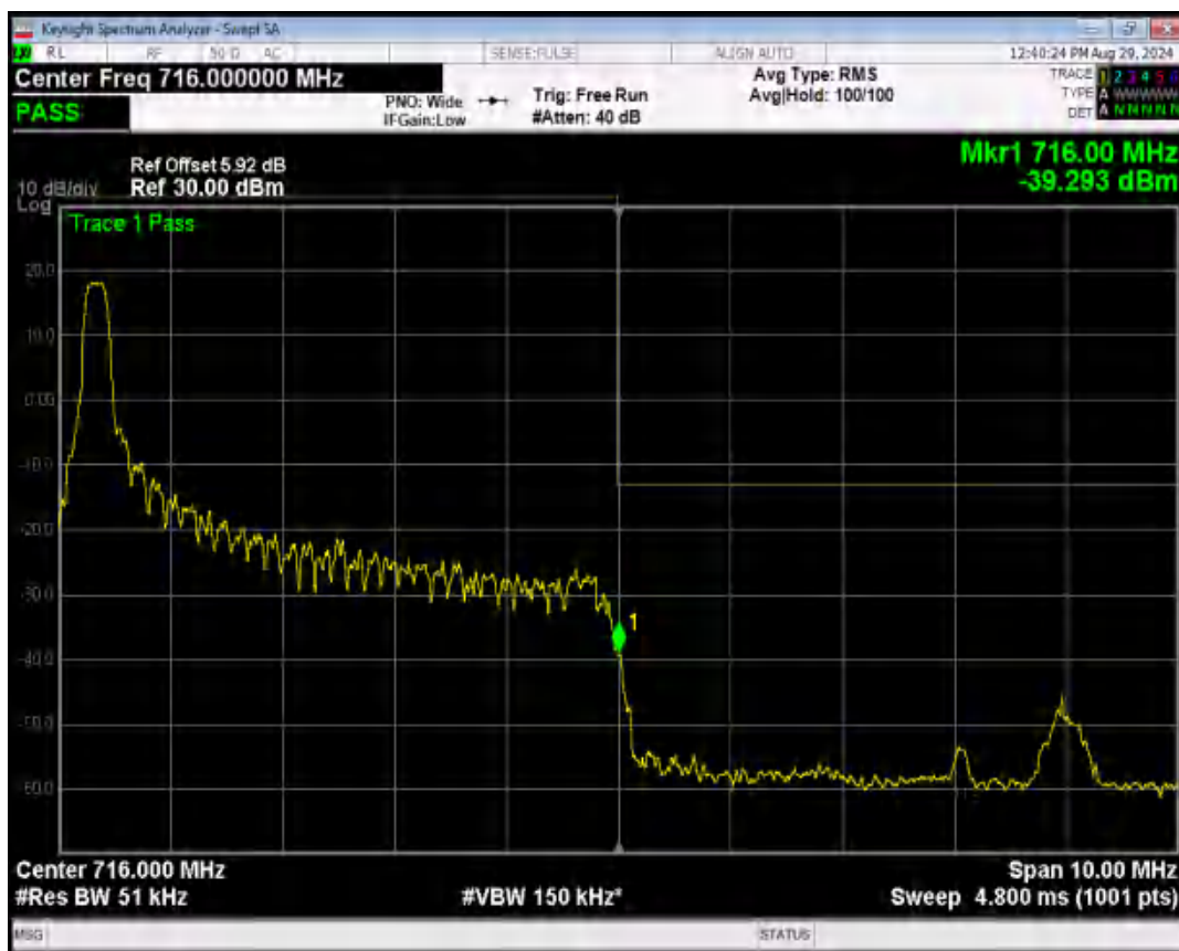
Band17 16QAM BW=5MHz Channel=23825 RB Size=1 Position=#Max
