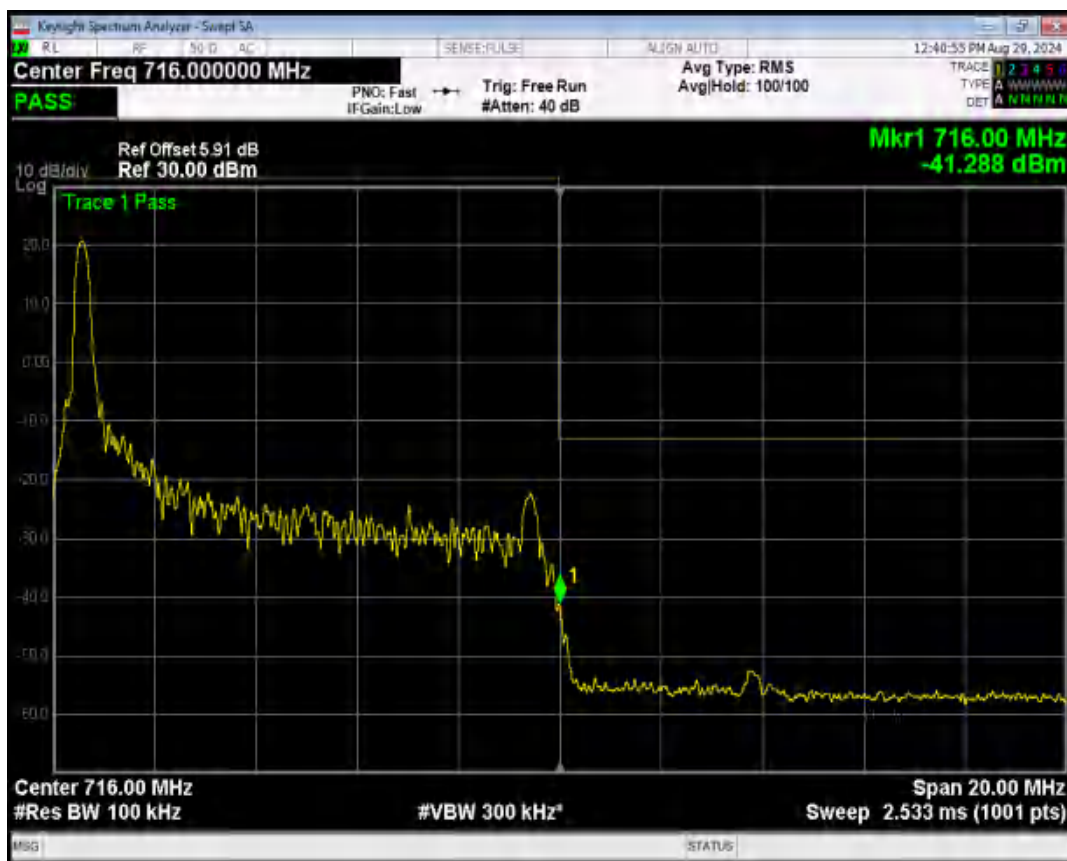
Band17 16QAM BW=10MHz Channel=23800 RB Size=1 Position=#Max
