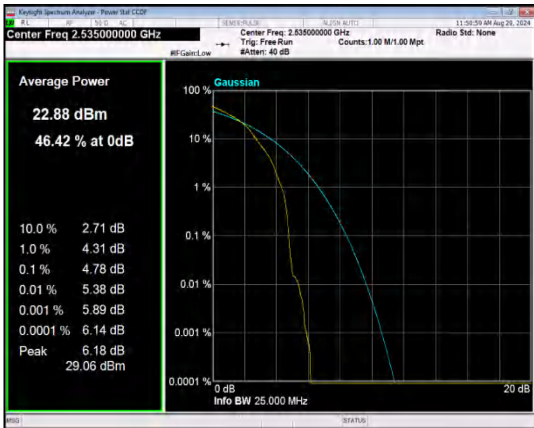
Band7 QPSK BW=20MHz Channel=21100 RB Size=1 Position=#0
