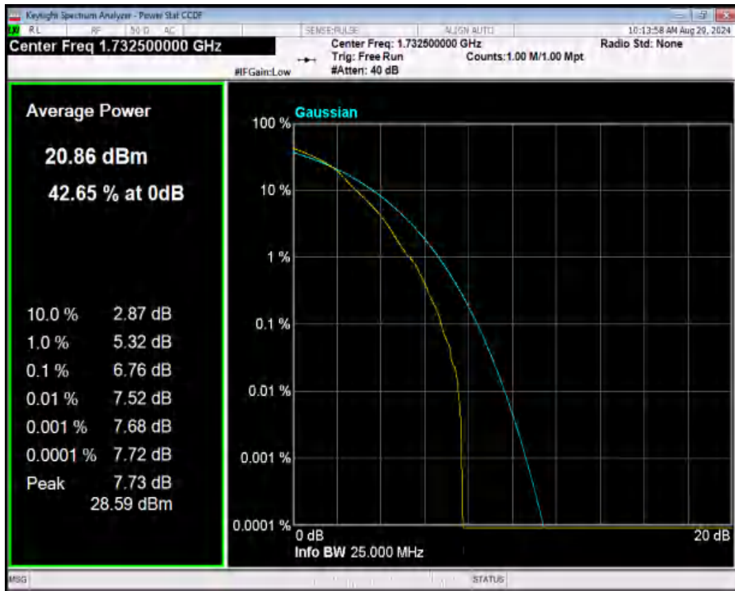
Band4 QPSK BW=5MHz Channel=20175 RB Size=1 Position=#0
