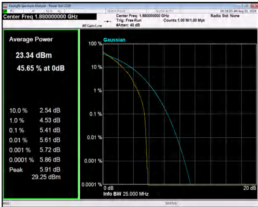
Band2 16QAM BW=15MHz Channel=18900 RB Size=1 Position=#0
