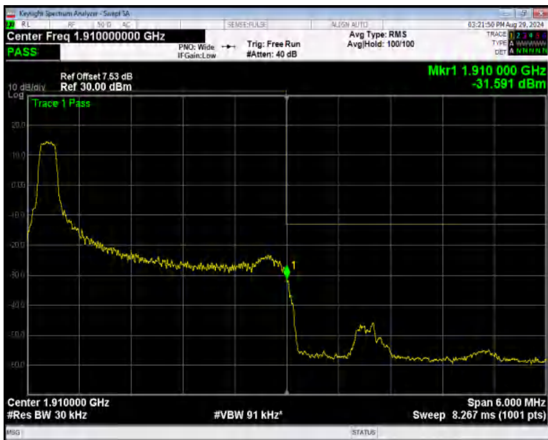
Band2 QPSK BW=3MHz Channel=19185 RB Size=1 Position=#Max
