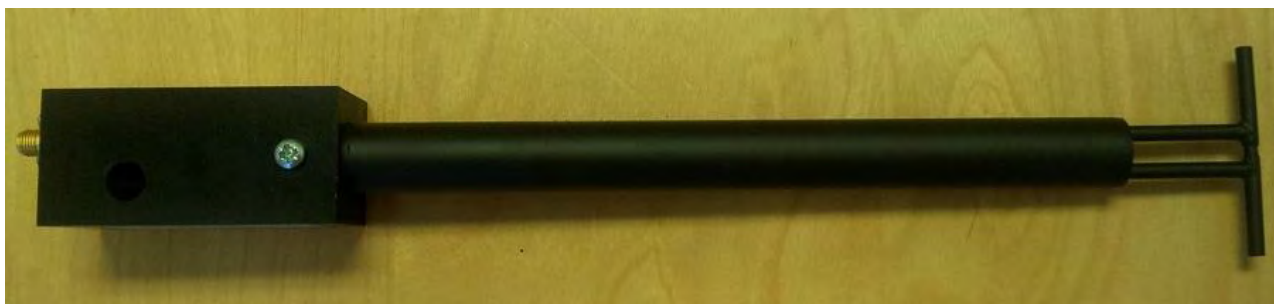
Figure 1 – MVG COMOSAR Validation Dipole
