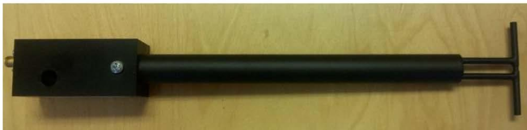
Figure 1 – MVG COMOSAR Validation Dipole
