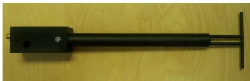
Figure 1 – MVG COMOSAR Validation Dipole
