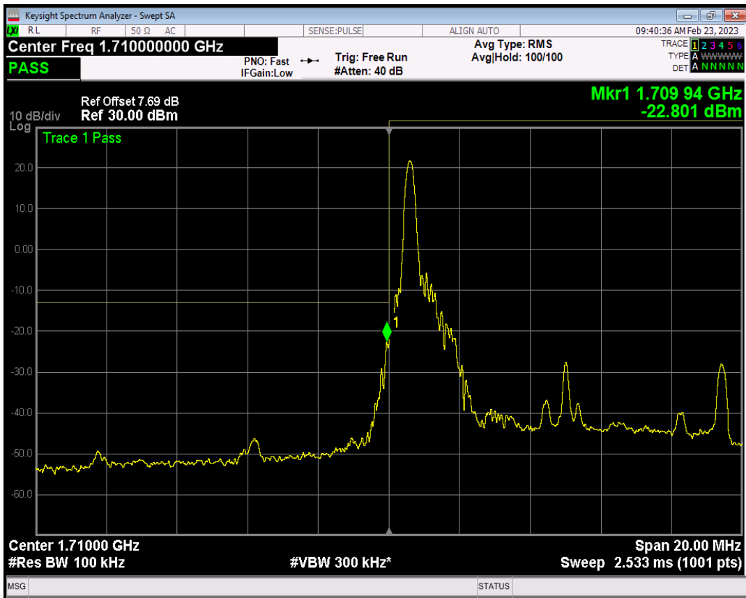
Band4 QPSK BW=10MHz Channel=20000 RB Size=1 Position=#Max
