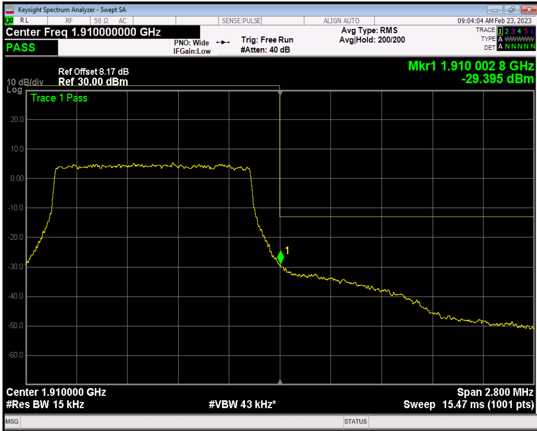
Band2 QPSK BW=3MHz Channel=18615 RB Size=1 Position=#0
