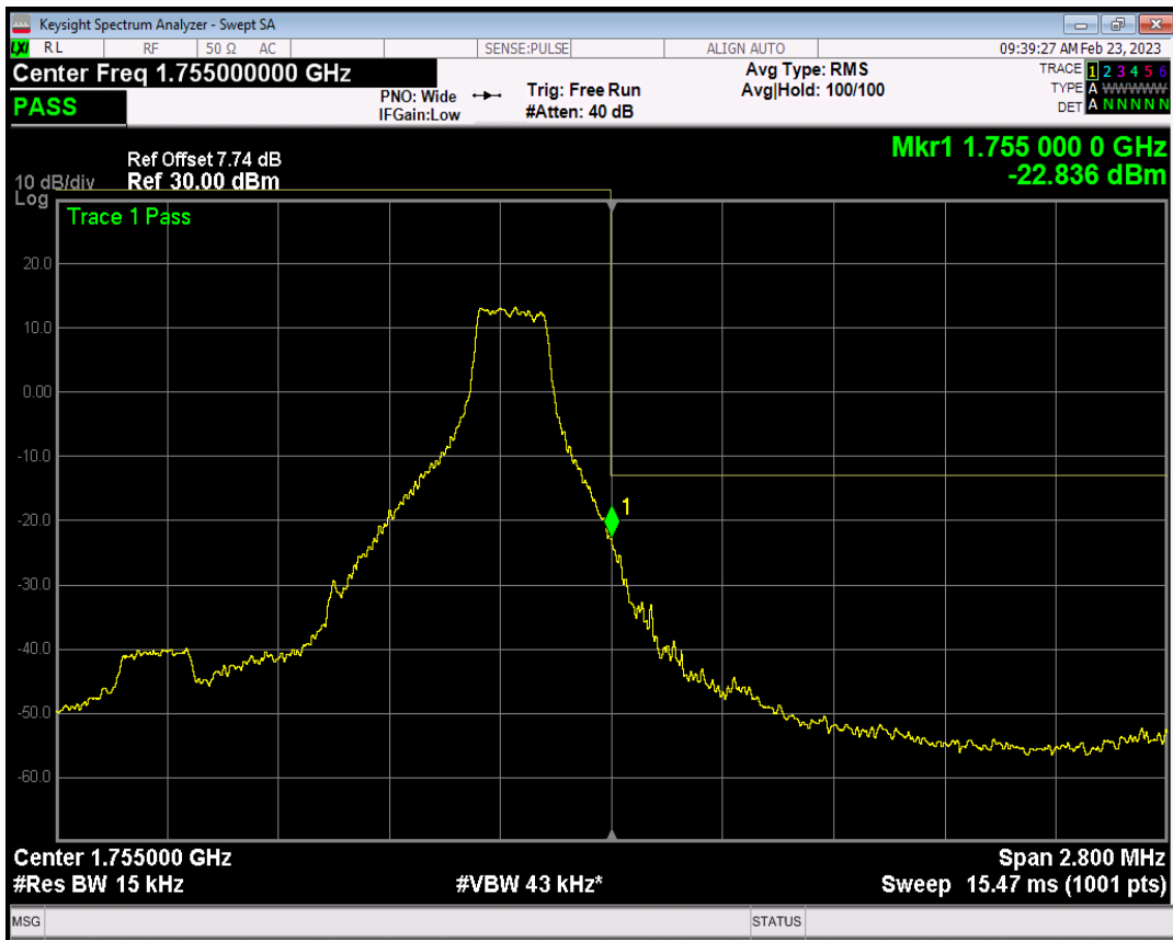
Band4 QAM16 BW=1.4MHz Channel=20393 RB Size=6 Position=#0
