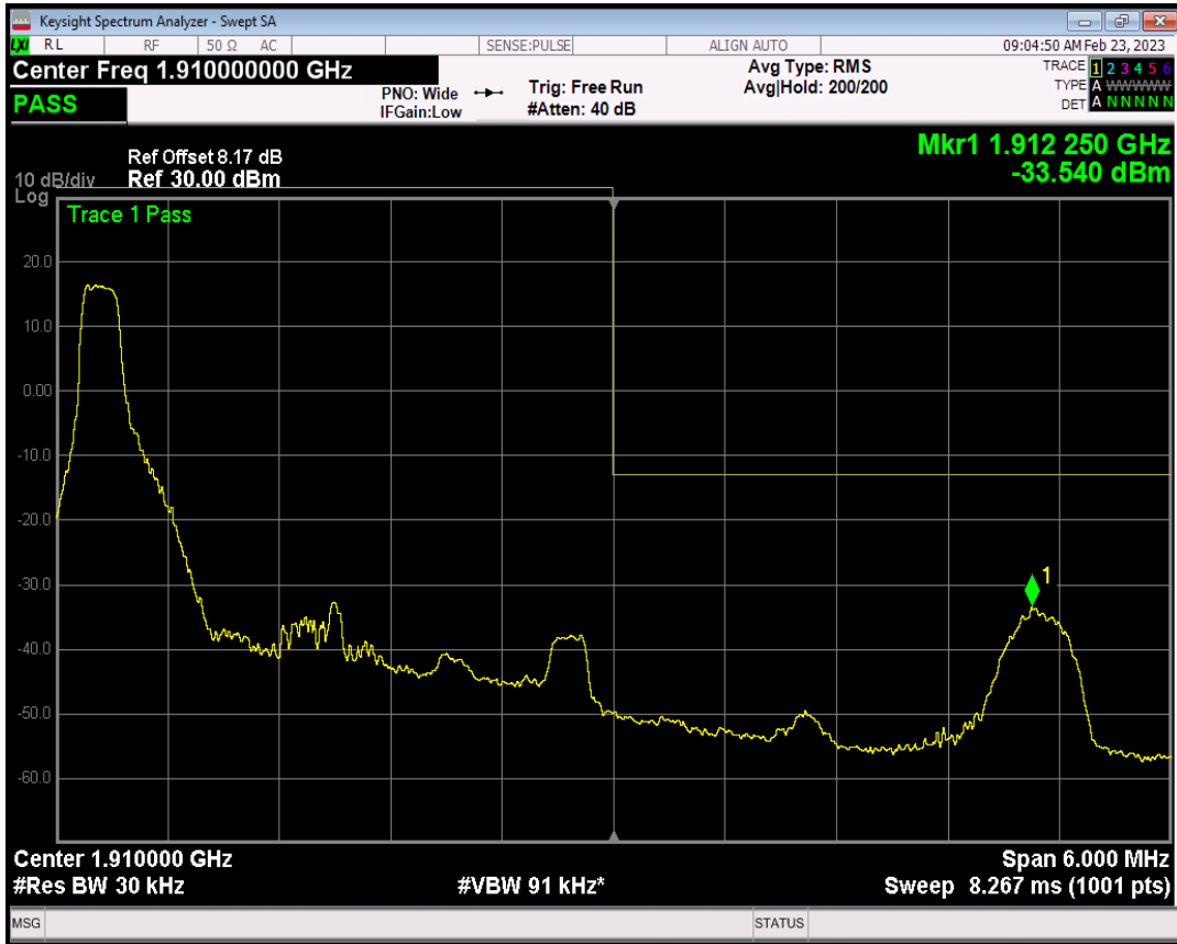
Band2 QAM16 BW=3MHz Channel=19185 RB Size=1 Position=#Max
