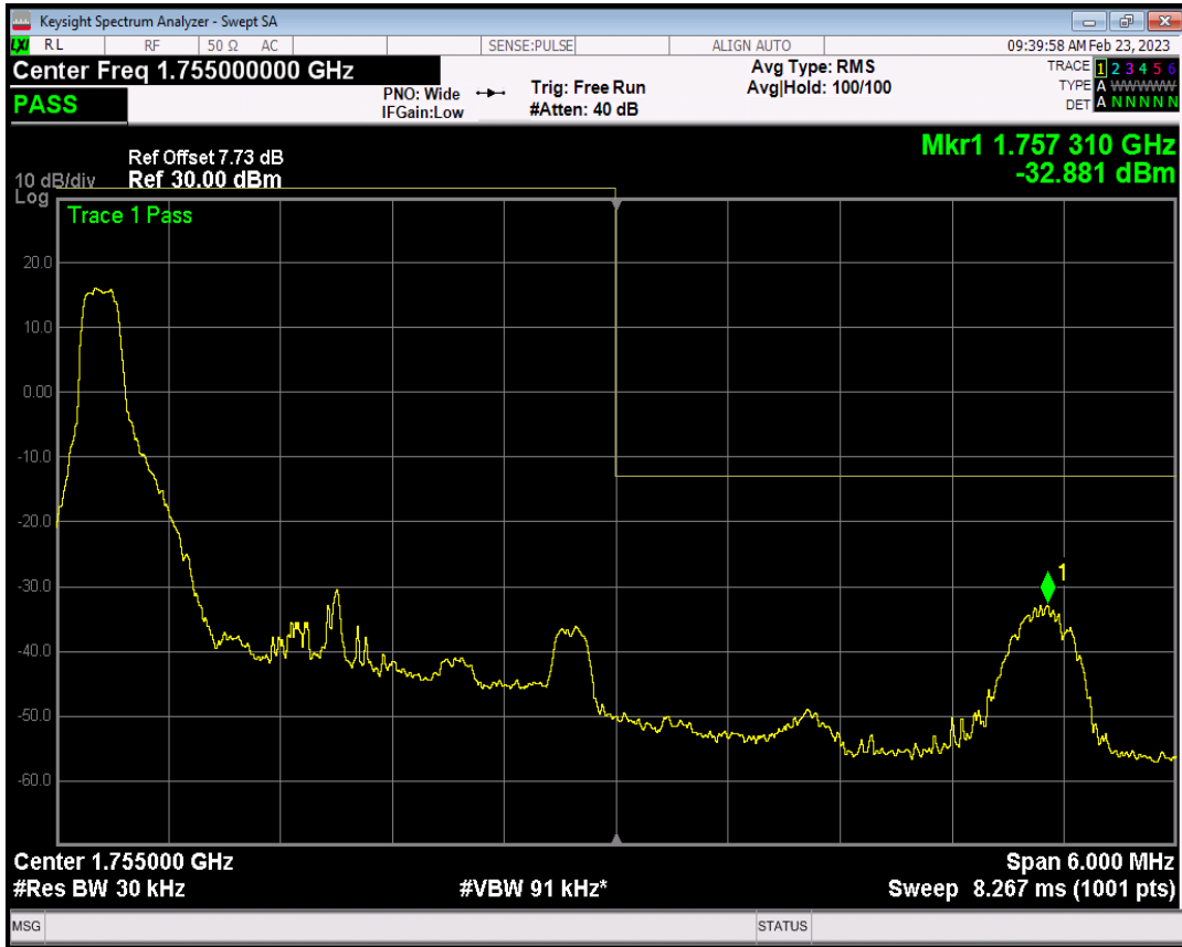
Band4 QAM16 BW=3MHz Channel=20385 RB Size=1 Position=#Max
