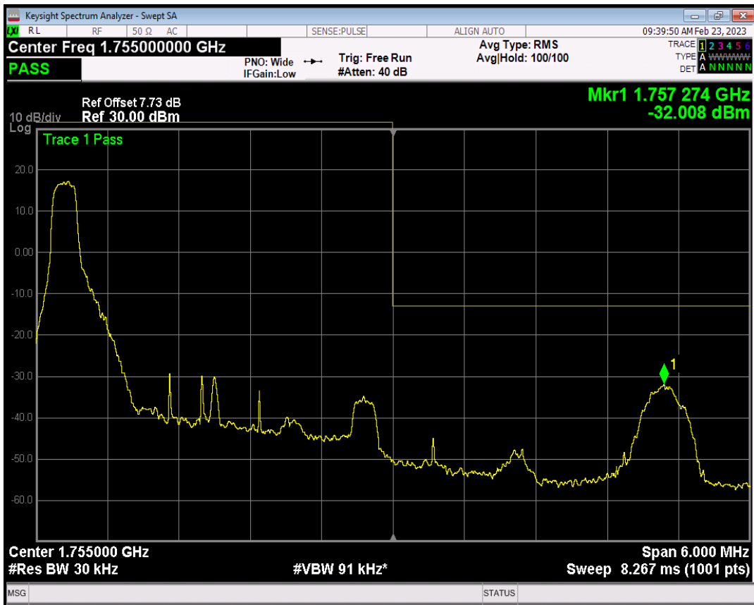
Band4 QPSK BW=3MHz Channel=20385 RB Size=1 Position=#Max
