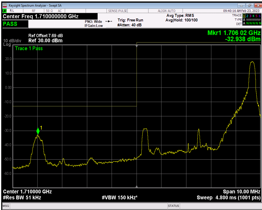
Band4 QAM16 BW=5MHz Channel=19975 RB Size=25 Position=#0
