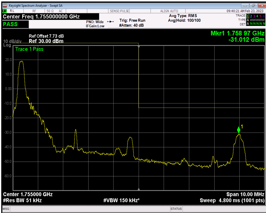
Band4 QPSK BW=5MHz Channel=20375 RB Size=1 Position=#Max
