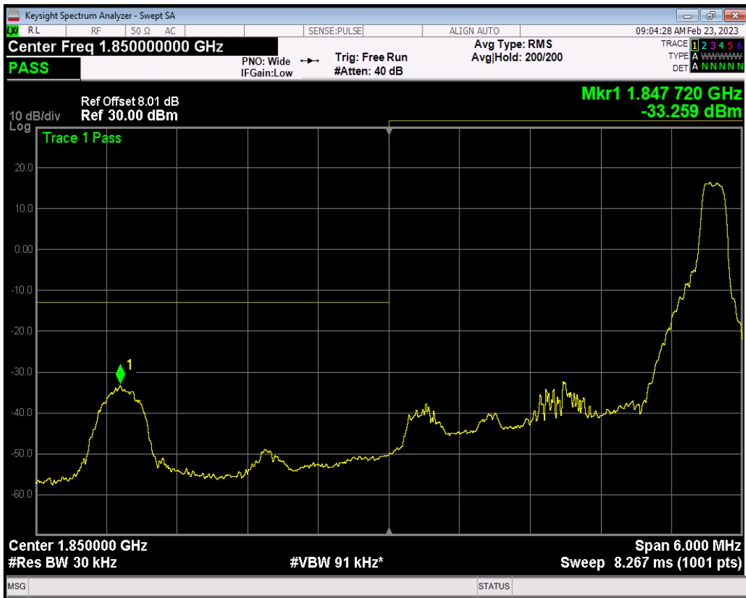
Band2 QAM16 BW=3MHz Channel=18615 RB Size=15 Position=#0
