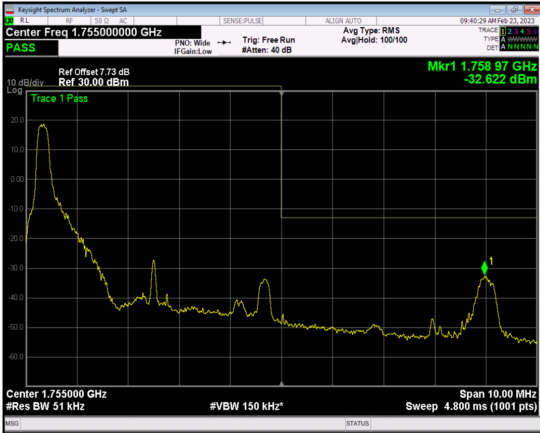
Band4 QAM16 BW=5MHz Channel=20375 RB Size=1 Position=#Max
