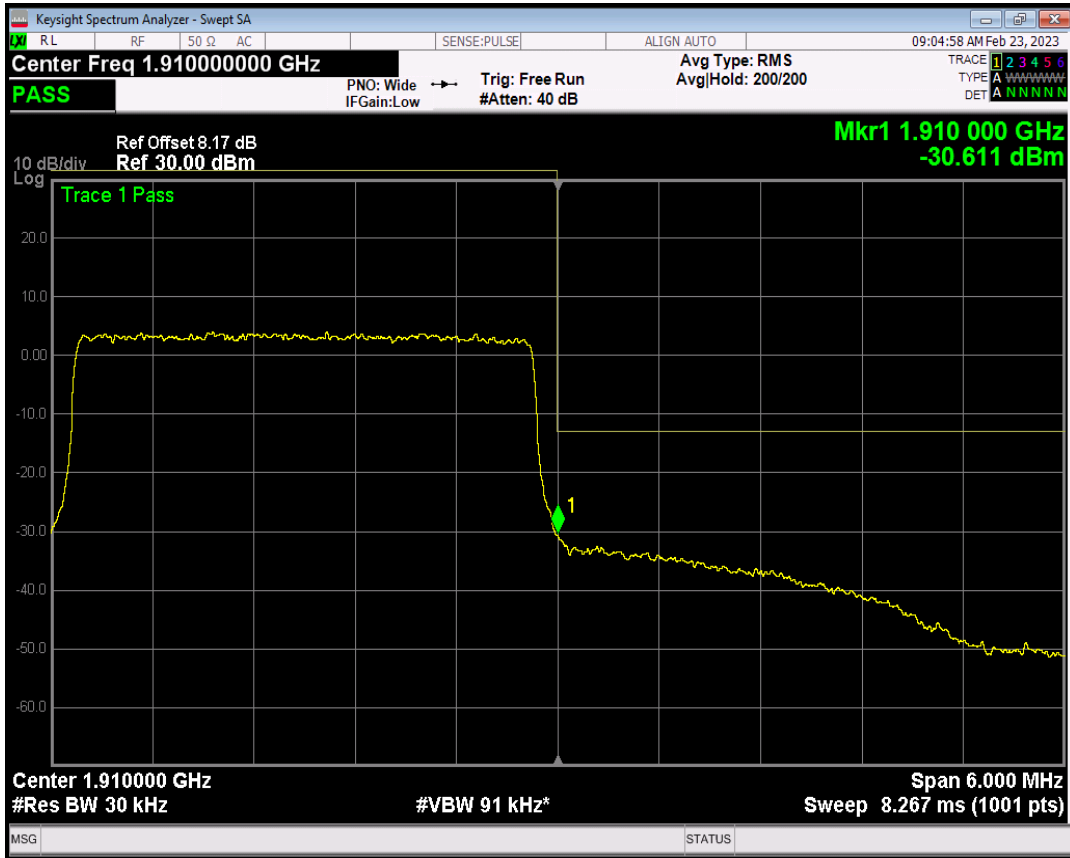
Band2 QPSK BW=5MHz Channel=18625 RB Size=1 Position=#Max
