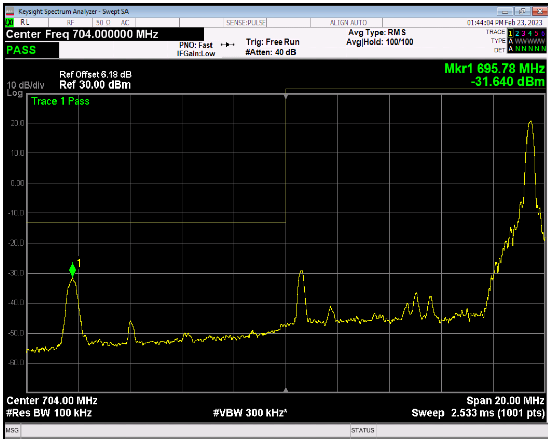
Band17 QAM16 BW=10MHz Channel=23780 RB Size=50 Position=#0
