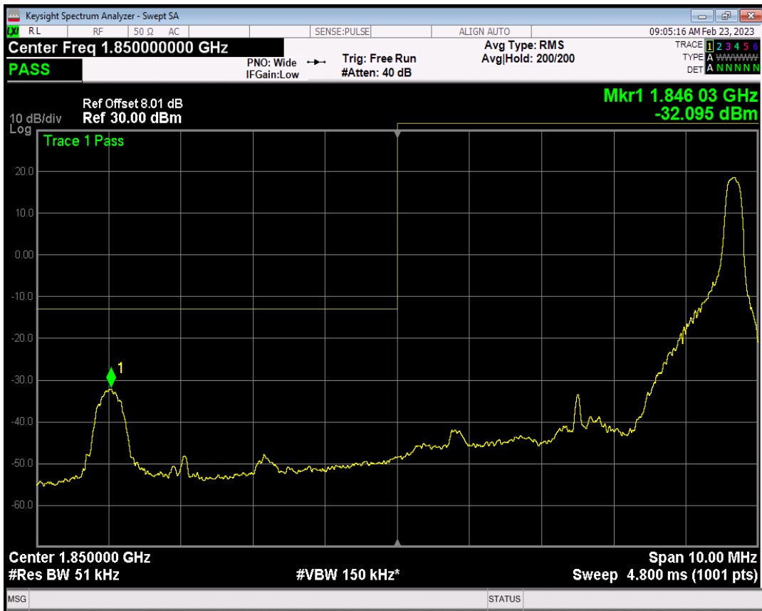
Band2 QAM16 BW=5MHz Channel=18625 RB Size=25 Position=#0
