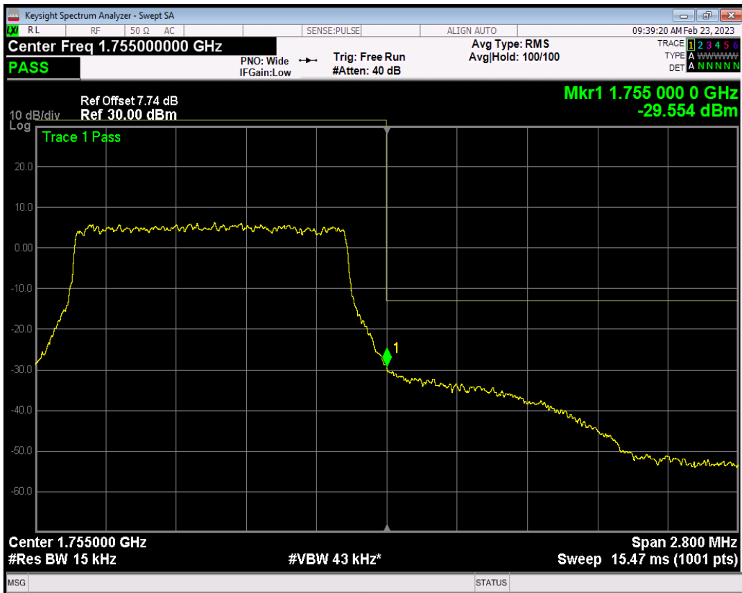
Band4 QAM16 BW=1.4MHz Channel=20393 RB Size=1 Position=#0
