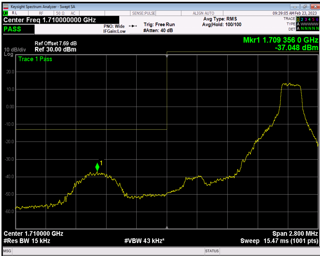
Band4 QAM16 BW=1.4MHz Channel=19957 RB Size=6 Position=#0
