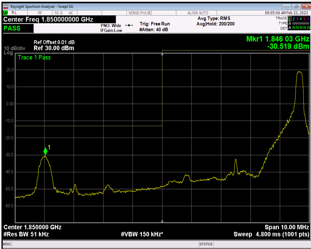
Band2 QPSK BW=5MHz Channel=18625 RB Size=1 Position=#0
