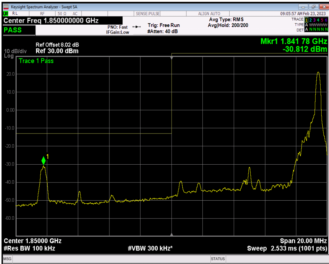
Band2 QAM16 BW=10MHz Channel=18650 RB Size=50 Position=#0
