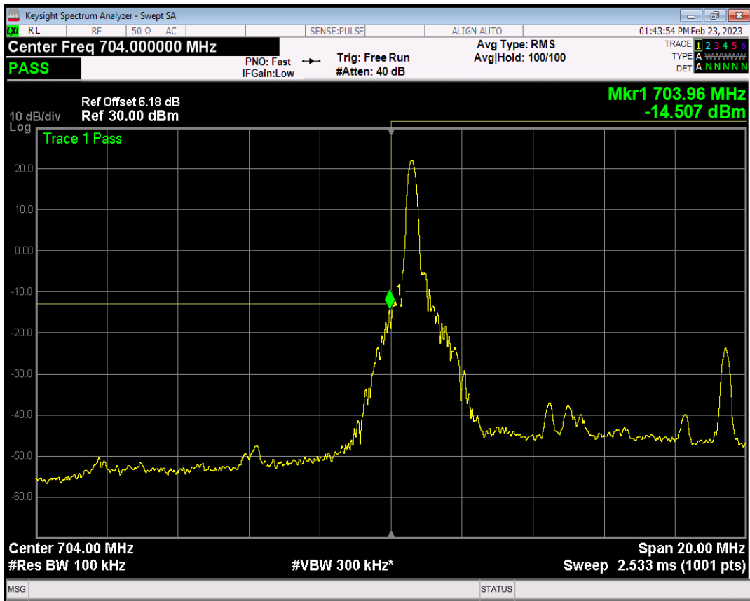
Band17 QPSK BW=10MHz Channel=23780 RB Size=1 Position=#Max
