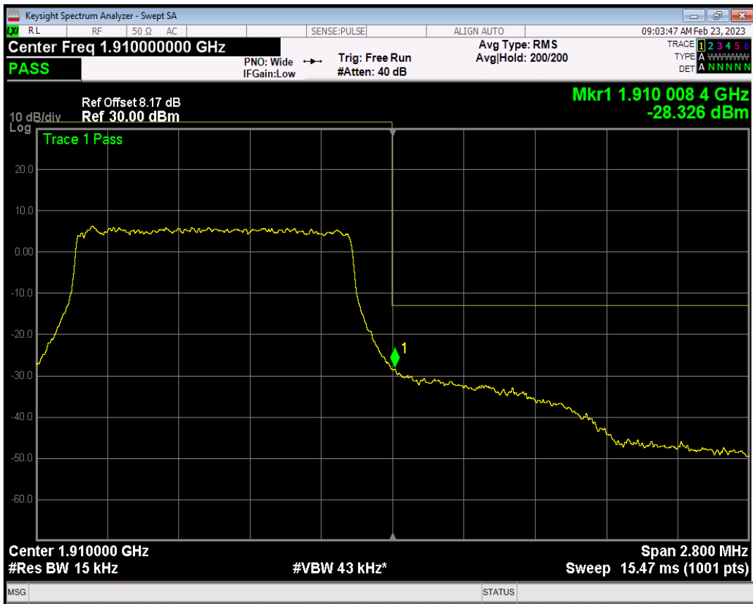
Band2 QAM16 BW=1.4MHz Channel=19193 RB Size=1 Position=#0
