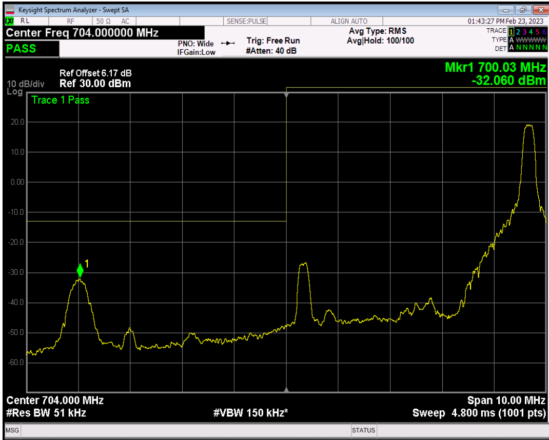
Band17 QPSK BW=5MHz Channel=23755 RB Size=25 Position=#0
