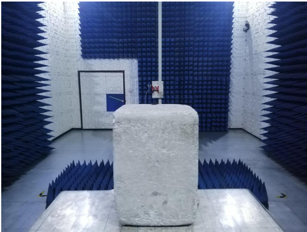
RADIATED EMISSION TEST SETUP ABOVE 1GHz
