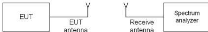
Figure 7.4.1 Occupied bandwidth test setup
