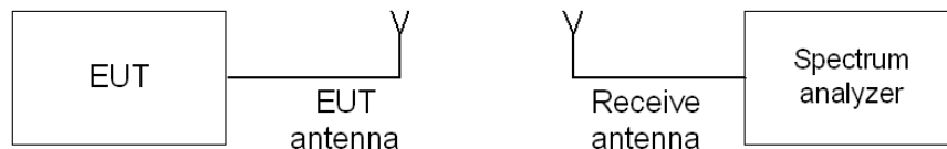
Figure 7.4.1 Occupied bandwidth test setup
