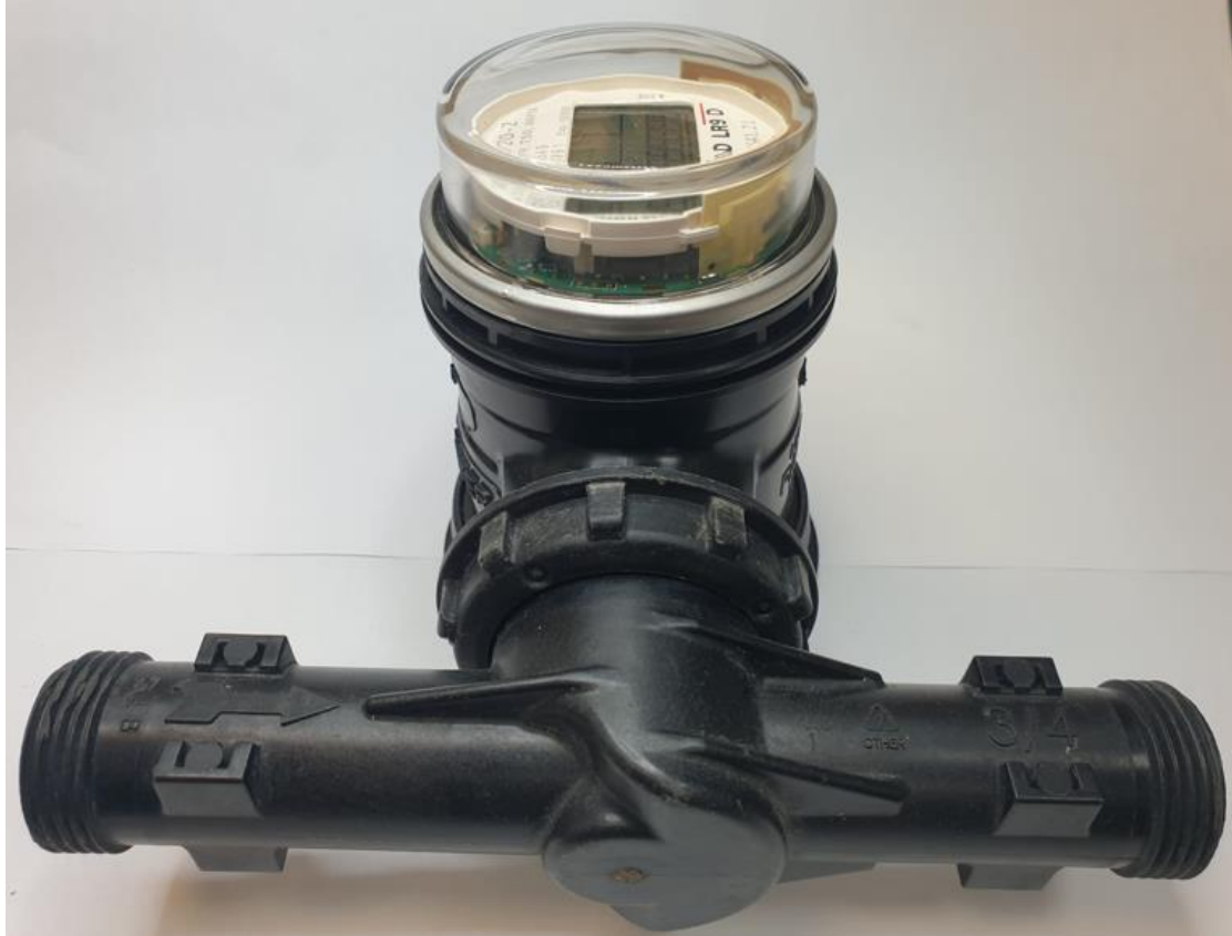
Photograph No.3 “INTERPRETER FAM LR9” water meter with cover removed
