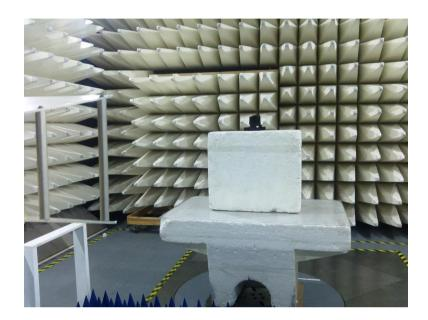
Photograph No.5 Setup for hopping parameters, OBW, power, power density, band edge emissions e measurements
