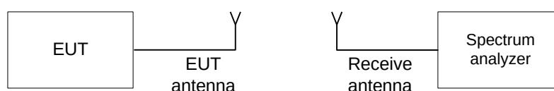
Figure 7.1.1 The 20 dB bandwidth test setup
