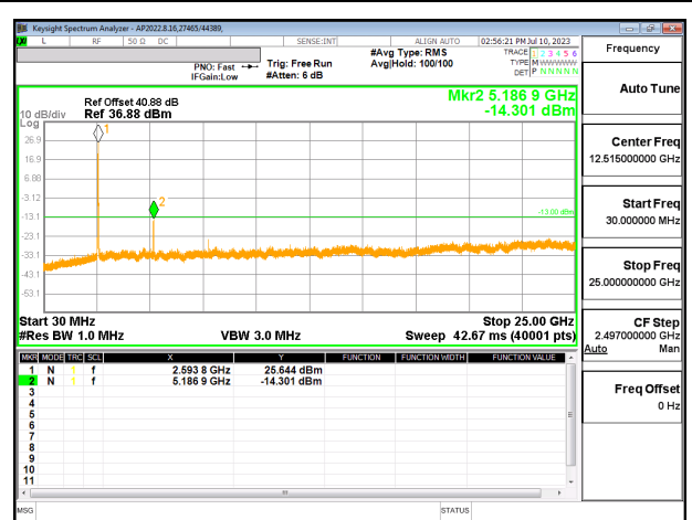
LTE41 20MHz QPSK MID Ch RB100-0
