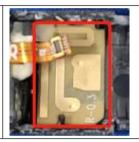
The antenna is FPC antenna. The best case gain of the antenna is 0.35 dBi.
