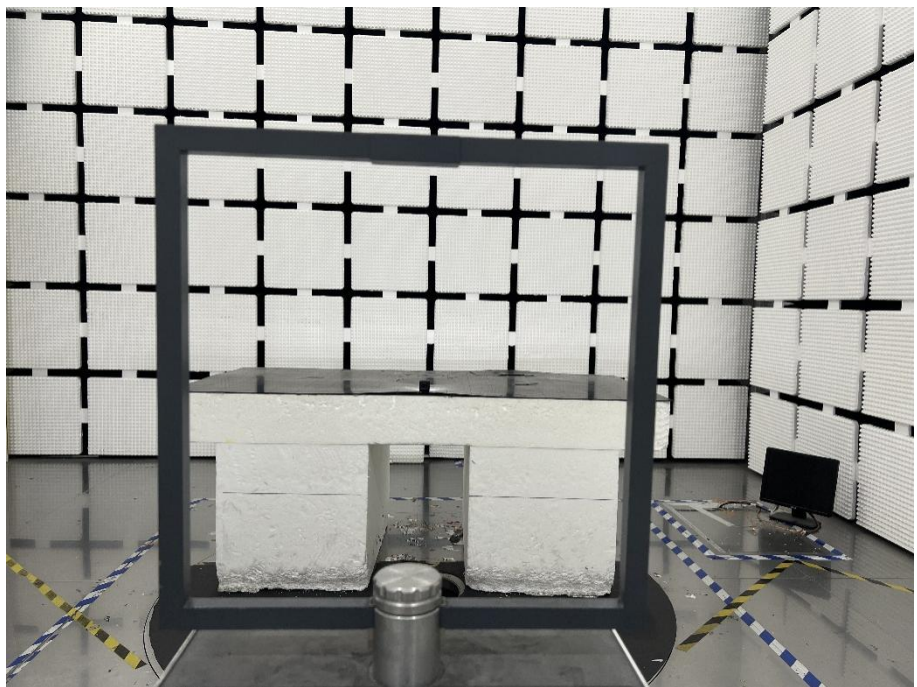
Radiation Emission Test Setup (Below 30MHz)
