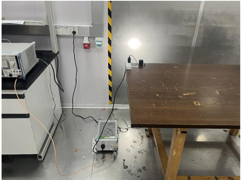
Conducted Emission Test Setup
