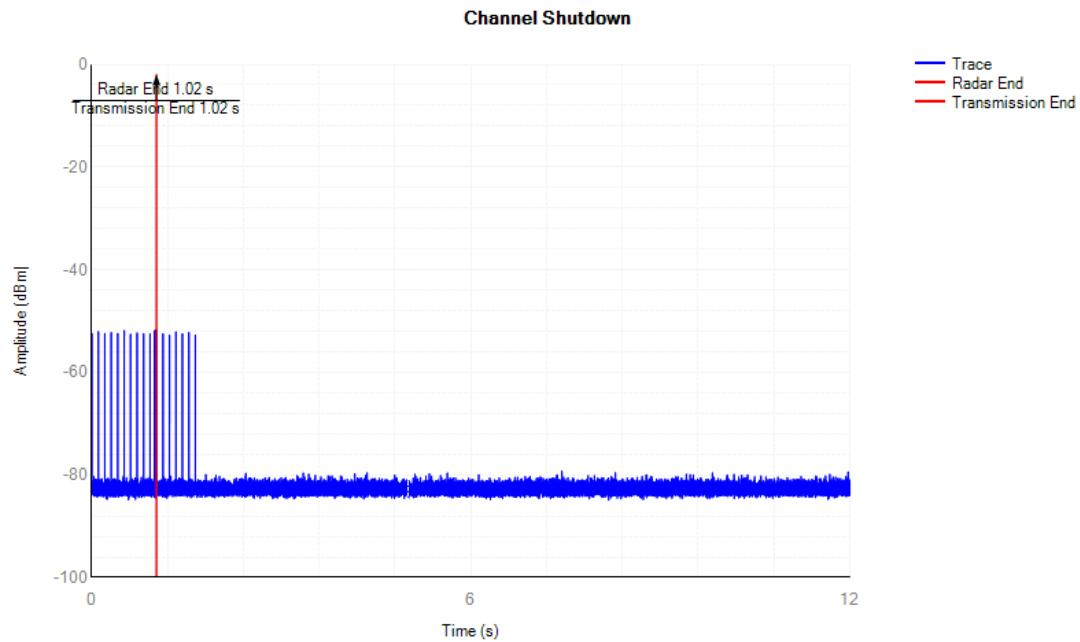
**Radar Type 0 Channel Closing Transmission**
