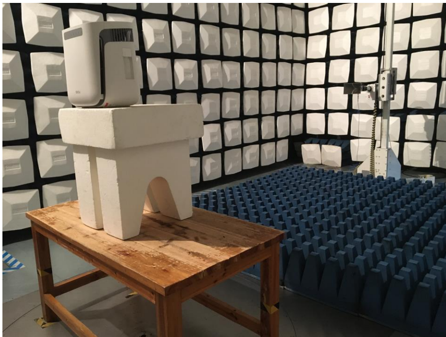
Test Setup For Radiated Emission (Above 1GHz)
