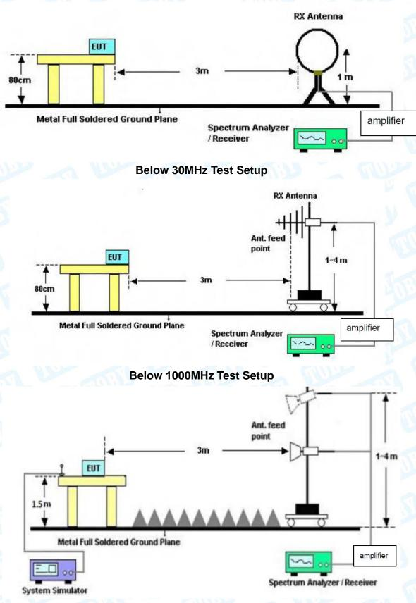
Above 1GHz Test Setup
