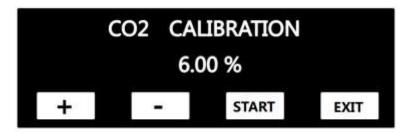
CO<sub>2</sub> Concentration Calibration Interface and Operation Instructions When MT300SP Is Not Connected
