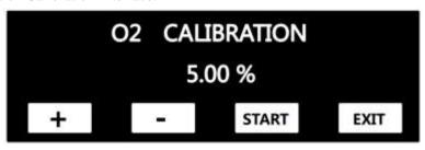
$\mathrm{O}_2$  Concentration Calibration Interface and Operation Instructions When MT300SP Is Not Connected
