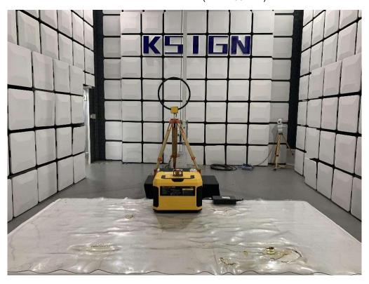
Radiated Measurement (Above 30MHz)
